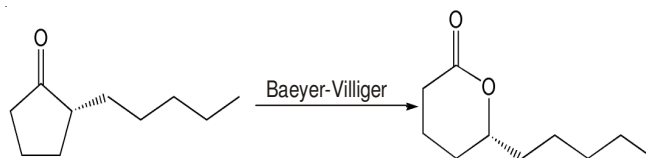
Fig. 2. Preparation of (R)- \delta -decalactone by the Baeyer-Villiger oxidation of (R)-2-alkylcyclopentanone with m -CPBA at room temperature
