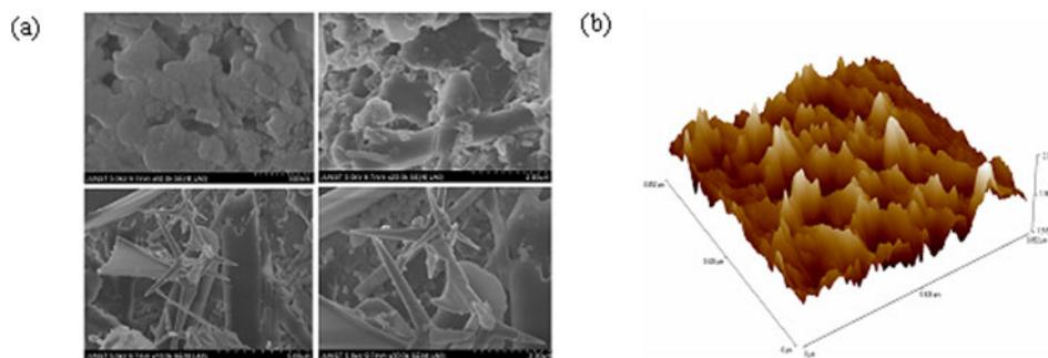
Figure 3. (Colour online) (a) SEM image of xerogel (at different scale bars) and (b) three-dimensional view of AFM image of xerogel from **1** and KF in DMSO:H<sub>2</sub>O (1:1, v/v).
