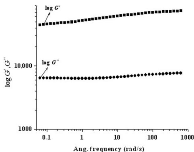
Figure 4. Variation of storage modulus ( $G'$ ) and loss modulus ( $G''$ ) with frequency.
