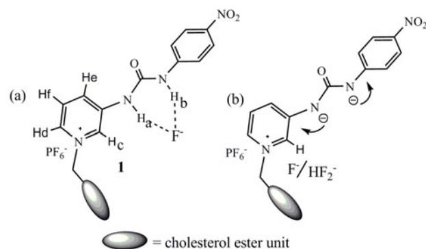
Figure 2. (Colour online) Suggested scheme for (a) hydrogen bonding and (b) deprotonation in **1** in the presence of  $\text{F}^-$ .
