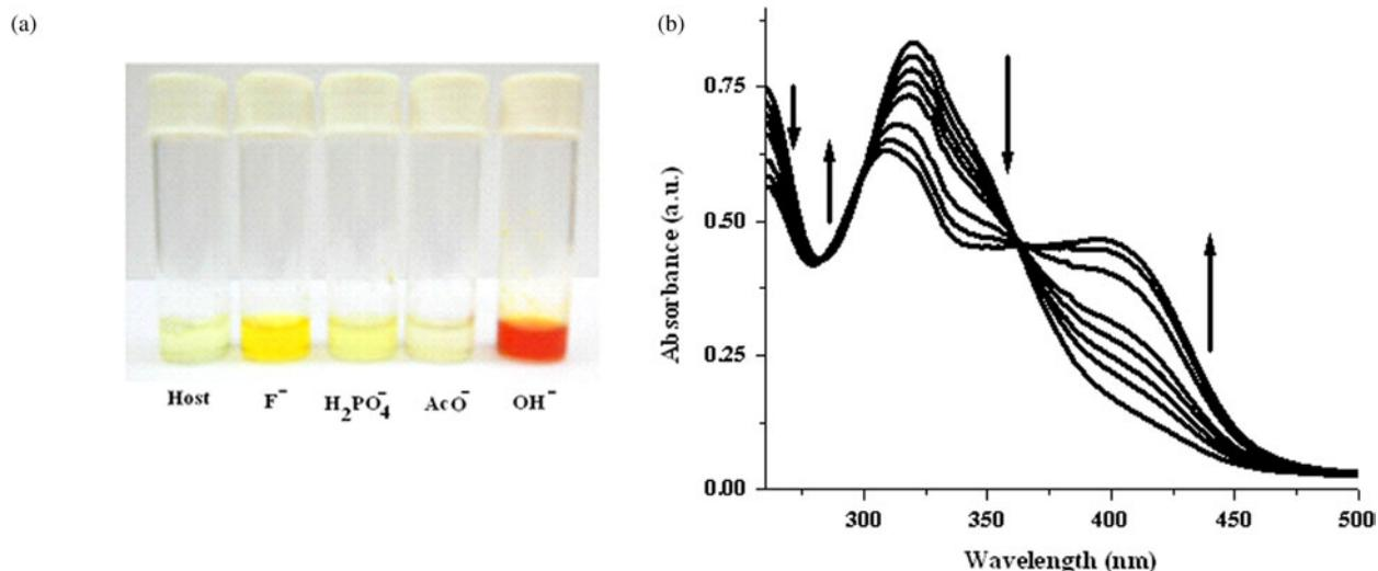
Figure 6. (Colour online) (a) Photographs of colour change of **1** ( $c = 1.5 \times 10^{-3}$  M) upon addition of TBAF, dihydrogenphosphate, acetate and hydroxide ( $c = 3.0 \times 10^{-3}$  M) in DMSO and (b) UV-vis titration spectra of **1** ( $c = 4.25 \times 10^{-5}$  M) with TBAF in DMSO.
