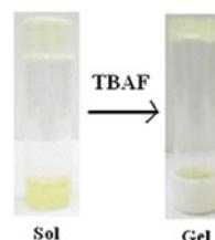
Figure 5. (Colour online) Photographs showing the phase changes of **1** in DMSO:H<sub>2</sub>O (1:1, v/v; 10 mg/ml) upon addition of 10 equiv. amounts of TBAF ( $c = 1.0 \times 10^{-3}$  M).
