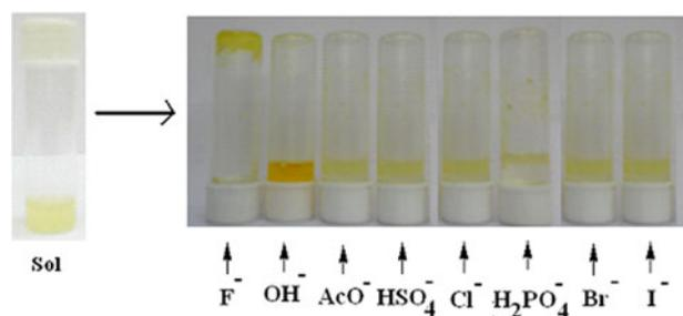
Figure 1. (Colour online) Photographs showing the phase changes of **1** in DMSO:H<sub>2</sub>O (1:1, v/v; 10 mg/ml) upon addition of 10 equiv. amounts of each anion of potassium salt ( $c = 1.0 \times 10^{-3}$  M).
