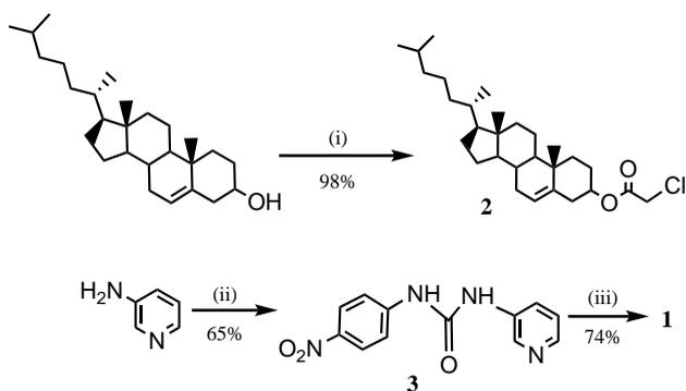
Scheme 1. (i) Chloroacetyl chloride, pyridine, dry  $\text{CH}_2\text{Cl}_2$ , room temperature (r.t.), 10 h; (ii) 4-nitroaniline, triphosgene,  $\text{Et}_3\text{N}$ , dry  $\text{CH}_2\text{Cl}_2$ , r.t., 24 h; (iii) a. 2, dry  $\text{CH}_3\text{CN}$ , reflux, 3 days, b.  $\text{NH}_4\text{PF}_6$ , DMF–water, r.t.,  $\frac{1}{2}$  h.
