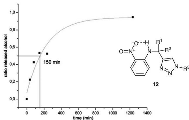
**Figure 2** Hydrogen bond in compound **12d** and hydrolysis determination at pH 4.3
