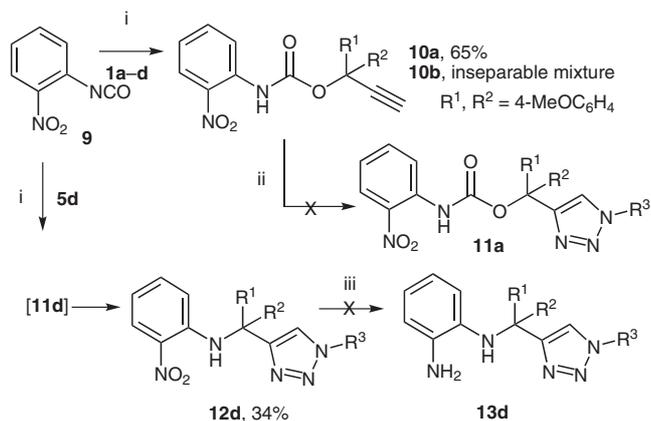
**Scheme 4** Reagents and conditions: (i) heptane, Et<sub>3</sub>N cat., reflux, 30 min; (ii) azide **3** (R<sup>3</sup>N<sub>3</sub>), CuI, solvents, 20 °C; (iii) SnCl<sub>2</sub>, EtOH.
