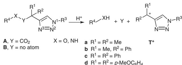
**Scheme 1** Principle of triazolyl-based acid-sensitive systems
