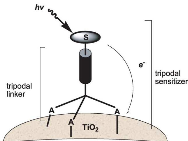
**Figure 1.** Schematic representation of the components of a tripodal sensitizer bound to a TiO<sub>2</sub> nanoparticle. These are: the sensitizing chromophore (S) and the tripodal linker, containing a rigid-rod bridge (b) and three anchoring groups (A).
