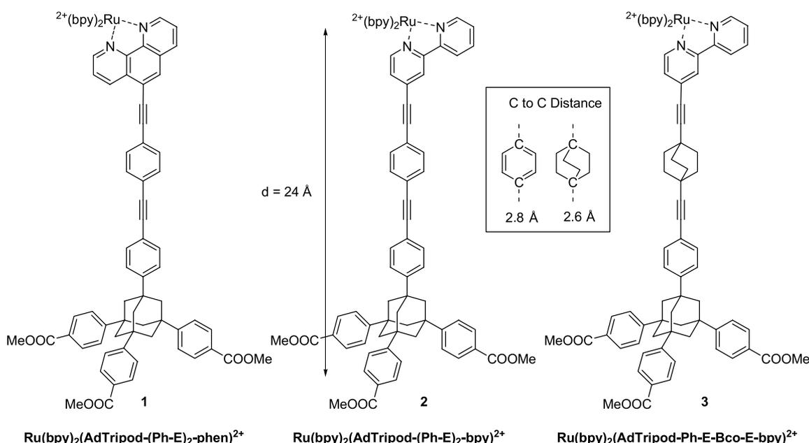
**Figure 2.** Tripodal sensitizers **1**, **2** and **3**. The counterion is PF<sub>6</sub><sup>-</sup> in all cases. Note the phen ligand in **1** and bpy ligand in **2**. Tripod **3** contains a Bco unit that retains the axial symmetry and has the same length as a Ph unit (inset). The distance ( $d$ ) of the Ru center to the footprint (the plane defined by the three surface-bound oxygen atoms) in **1–3** is 24 Å.<sup>7</sup>
