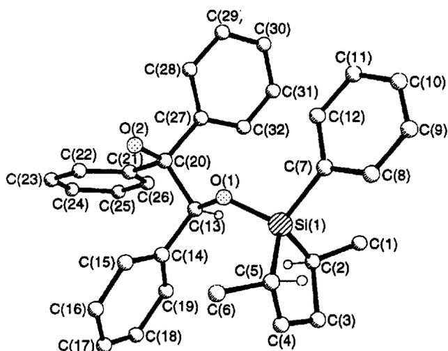
**Fig. 2** Molecular structure of the (S,S)-silyl ether 17 derived from (S)-TPED (only selected hydrogen atoms are shown). Selected bond lengths (Å) and bond or torsion angles (°) are as follows: Si(1)–O(1) 1.649(4), Si(1)–C(2) 1.853(9), Si(1)–C(5) 1.884(14), Si(1)–C(7) 1.885(8), Si(1)–O(1)–C(13) 128.5(3), C(2)–Si(1)–C(5) 98.7(5), C(7)–Si(1)–O(1) 105.1(3), C(2)–C(3)–C(4)–C(5) 39.3.
