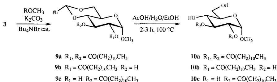
**Scheme 5.****Table 4.** Transesterification of **3** (705 mg, 2.5 mmol) with methyl laurate in basic medium ( $K_2CO_3$ ) in the presence of  $Bu_4NBr$  (4%) and DMF (2 mL, 10 equiv). Microwave power:  $P = 150\text{--}15\text{ W}$ .
