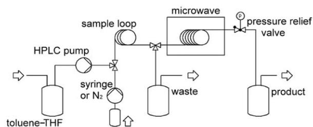
**Figure 1** Continuous-flow reactor setup: For the optimization procedure the sample is injected by a syringe into the sample loop outside the microwave oven. For the preparative use, the sample loop is removed, and the reaction mixture is introduced directly by the HPLC pump
