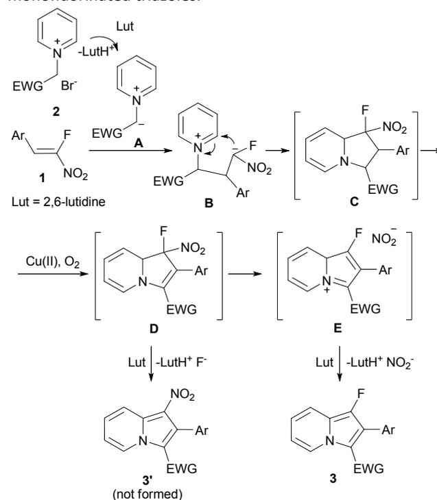
Scheme 5. Proposed mechanism for the synthesis of indolizines **3**.
