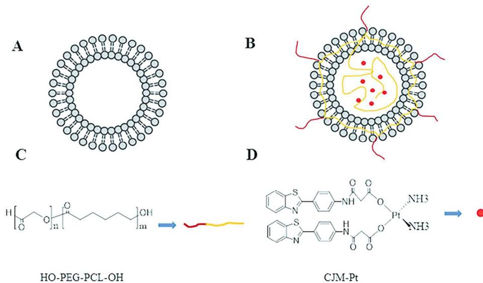
Fig. 2. Pure phosphatide liposomes (A). CJM-Pt loaded liposomes (B). HO-PEG-PCL-OH (C) and CJM-Pt (D).
