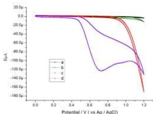
**Figure 1.** Cyclic voltammograms recorded in *n*-Me<sub>4</sub>NBF<sub>4</sub>/MeOH (0.1 M): (a) blank, (b) **1a** (0.006 M), (c) NaOMe (0.015M), (d) **1a** (0.006 M) + NaOMe (0.015 M).
