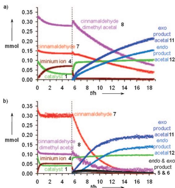
**Figure 2.** Diels–Alder reaction between cinnamaldehyde and cyclopentadiene catalyzed by 1-HCl in a)  $\text{CD}_3\text{OD}$  and b)  $\text{CD}_3\text{OD}/\text{D}_2\text{O}$  (19:1).
