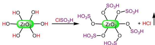
**Scheme 1** Schematic representation of the synthesis of zirconia sulfuric acid (ZrSA)
