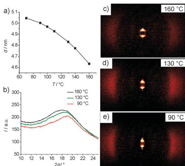
**Fig. 3** XRD data of compound **1b**: (a) dependence of layer distance  $d$  and (b) shape of the diffuse wide angle scattering on temperature; (c–e) diffraction pattern of a surface aligned sample (after subtraction of the scattering pattern in the Iso phase at  $T = 178$  °C); (c) SmA at  $T = 160$  °C; (d) SmAP<sub>R</sub> at  $T = 130$  °C; (e) SmAP<sub>A</sub> at  $T = 90$  °C (for original patterns, see Fig. S2, XRD patterns of compound **1a** are shown in Fig. S1, ESI†).
