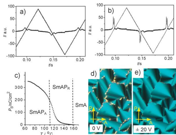
**Fig. 4** Electrooptical investigation of compound **1b**: (a,b) Switching current response in a 6 μm ITO cell (18  $V_{pp}$ , 10 Hz, 5 kΩ) on applying a triangular wave field; (a) in the SmAP<sub>R</sub> phase at  $T = 112$  °C; (b) in the SmAP<sub>A</sub> phase at  $T = 105$  °C; (c) temperature dependence of the spontaneous polarization (9.5 μm, 20 V, 100 Hz); (d,e) textures of the SmAP<sub>R</sub> phase at 153 °C depending on applied voltage.
