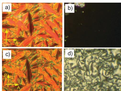
**Fig. 1** Changes of the textures of compound **1a** at the SmA-to-SmAP<sub>A</sub> phase transition (crossed polarizers); (a,b) SmA phase at *T* = 130 °C; (c,d) SmAP<sub>A</sub> phase at *T* = 100 °C; (a,c) fan-like texture; (b,d) homeotropically aligned sample.
