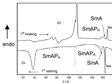
**Fig. 2** DSC heating and cooling curves (10 K min<sup>-1</sup>) of compound **1b**.
