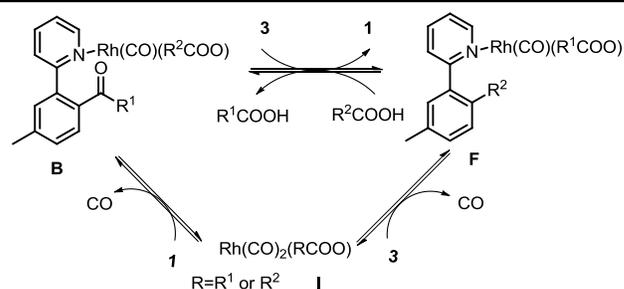
Figure 7. Ligand exchange of catalyst and resting states of catalyst
