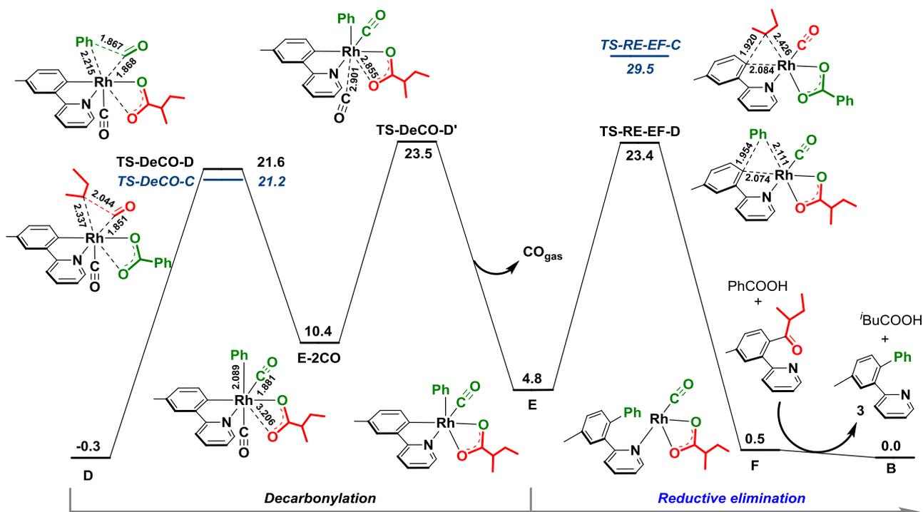
Figure 12. The decarbonylation, CO emission and reductive elimination steps of intermediate D. The decarbonylation and reductive elimination transition states for intermediate C were also shown (in italic). The selected bond lengths are in angstroms, and the relative free energies in chlorobenzene Gsol (413.15 K, 1.0 atm) are in kcal/mol. Calculated at M06/6-31+G\*\*/SDD level.
