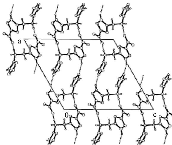
**Fig. 2.** Crystal packing of molecules of 1-[2-(3-nitro-1*H*-1,2,4-triazol-1-yl)ethyl]-1*H*-tetrazole (**III**). Hydrogen bonds are shown by dashed lines.
