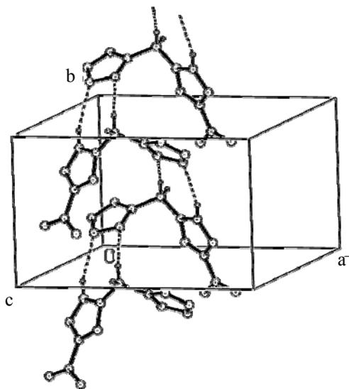
**Fig. 4.** Polymer chain bound by hydrogen bonds in the crystal structure of 2-*tert*-butyl-5-(3-nitro-1*H*-1,2,4-triazol-1-ylmethyl)-2*H*-tetrazole (**V**). *tert*-Butyl groups are not shown.
