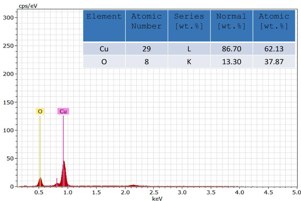
Fig. 3. EDAX spectrum of CuO nanostructures synthesized by *S. glauca* leaf extract. Inset: Table shows weight percentage of Cu and O atoms.
