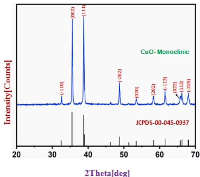
Fig. 1. XRD pattern of CuO nanostructures synthesized by *S. glauca* leaf extract.
