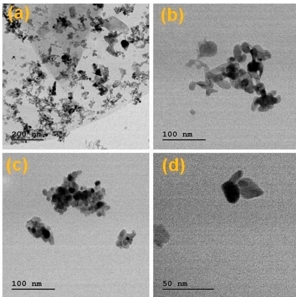
Fig. 4. TEM images of (a) 200 nm, (b,c) 100 nm, and (d) 50 nm CuO nanostructures synthesized by *S. glauca* leaf extract.
