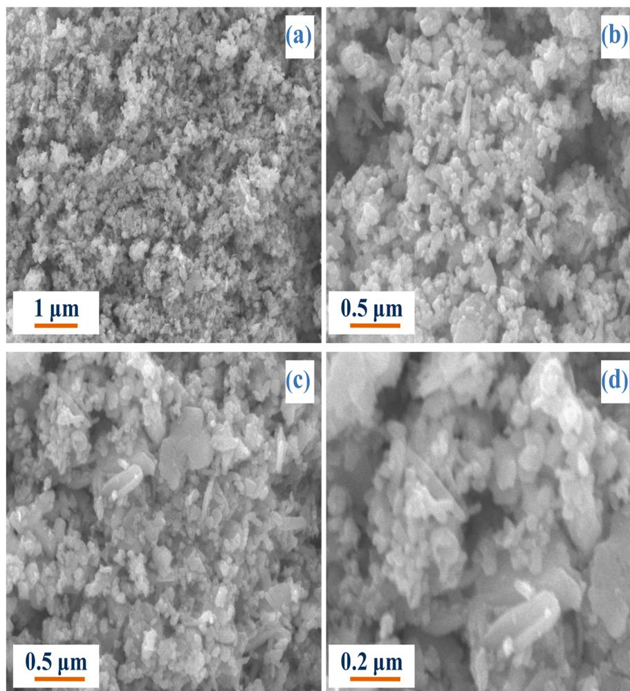
Fig. 2. SEM images of (a) 1  $\mu$ m, (b, c) 0.5  $\mu$ m, and (d) 0.2  $\mu$ m CuO nanostructures synthesized by *S. glauca* leaf extract.
