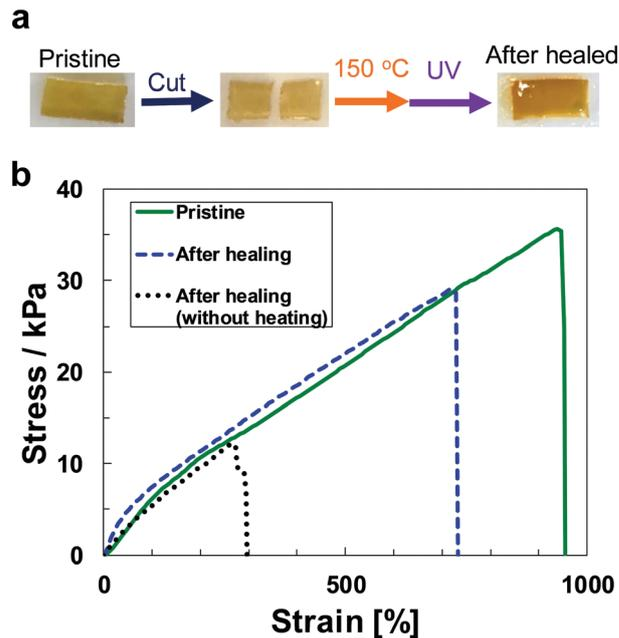
Fig. 4 (a) Photographic images of the pristine (left), cut (centre), and healed (right) 10 wt% tetraPEG–Ant ion gels. The cut ion gel pieces were re-contacted and healed by heating at 150 °C for 10 h and by UV irradiation overnight under an argon atmosphere. (b) Stress–strain curves for the pristine ion gel (green solid line), the healed ion gel by heating and UV irradiation (blue dashed line) and the healed ion gel only by UV irradiation (black dotted line).
