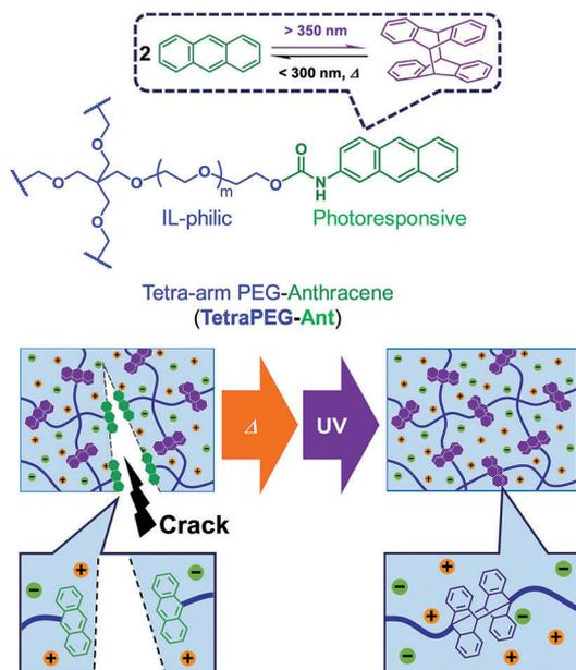
Fig. 1 The chemical structure of tetraPEG–Ant and a conceptual illustration of photohealing of the tetraPEG–Ant ion gel.
