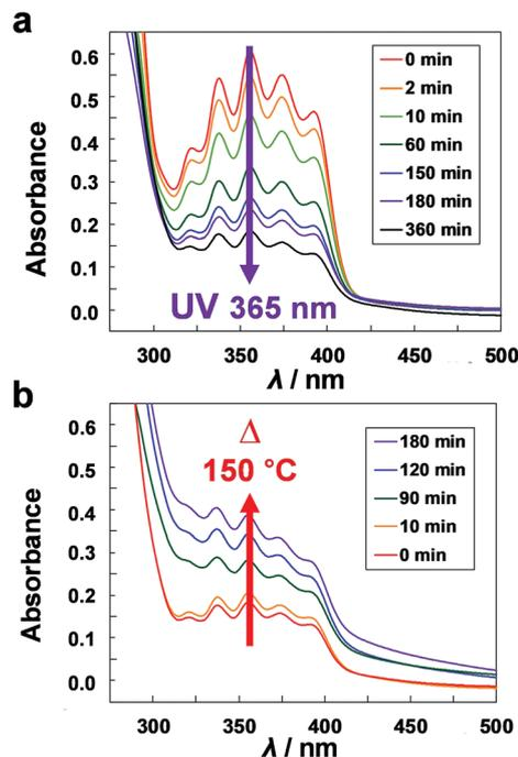
Fig. 2 Variation in the UV-vis spectra for a 1 wt% tetraPEG–Ant solution in  $[\text{C}_2\text{mim}][\text{NTf}_2]$  with time (a) under UV light ( $\lambda = 365$  nm) at room temperature, and (b) upon heating at 150 °C following UV irradiation.
