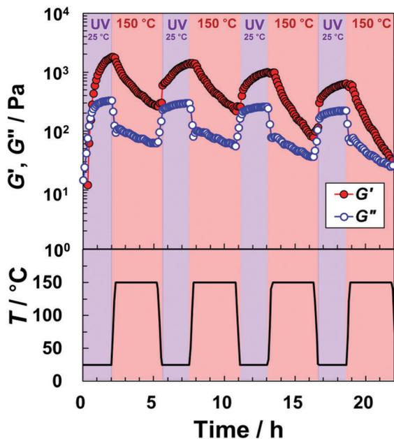
Fig. 3 Variation in  $G'$  and  $G''$  for a 10 wt% solution of tetraPEG–Ant in  $[\text{C}_2\text{mim}][\text{NTf}_2]$  as a function of time under alternating UV irradiation at 365 nm (2 h) and heating at 150 °C (3 h) at a frequency = 1 Hz and strain amplitude = 1%.
