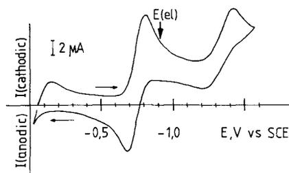
**Figure 2.** Cyclic voltammogram of lumiflavin (**1a**) in HMPT. Supporting electrolyte, tetra-butylammonium tetrafluoroborate.  $E_{(el)}$  indicates the voltage for electrolysis (cf. Fig. 5).
