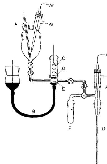
**Figure 3.** Design of the electrolysis cell for external reductive radical generation. A, solution storage vessel with silver wire pseudo reference electrode; B, mercury working electrode; C, platinum auxiliary electrode; D, glass frit; E, electrochemical cell with magnetic stirring bar; F, waste tube; G, sample tube.
