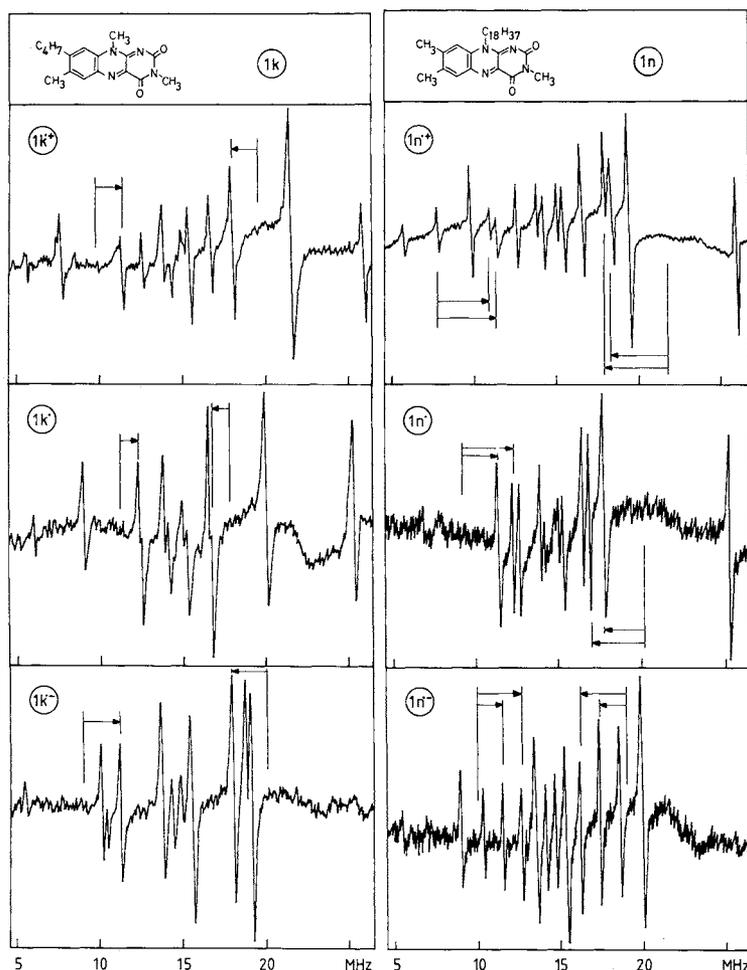
**Figure 6.** ENDOR spectra of the radicals from 8-normethyl-8-butylumiflavin (**1k**, left) and 10-normethyl-10-octadecyllumiflavin (**1n**, right) in their different protonation states. It should be noted that the  $\beta$ -proton resonances of the octadecyl substituent in the 10-position are significantly split, whereas those of the substituent in the 8-position are not.
