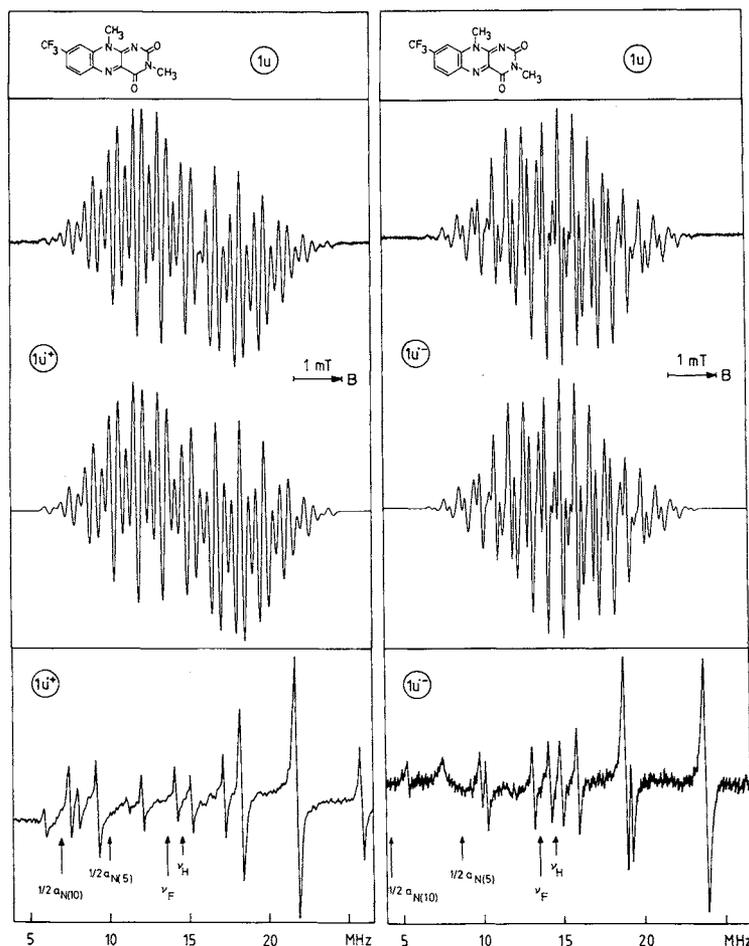
**Figure 4.** Experimental (top) and simulated (centre) EPR and ENDOR (bottom) spectra of the radical cation (left) and anion (right) of 3,10-dimethyl-8-(trifluoromethyl)isoalloxazine (**1u**) in toluene-trifluoroacetic acid and methylene chloride, respectively.
