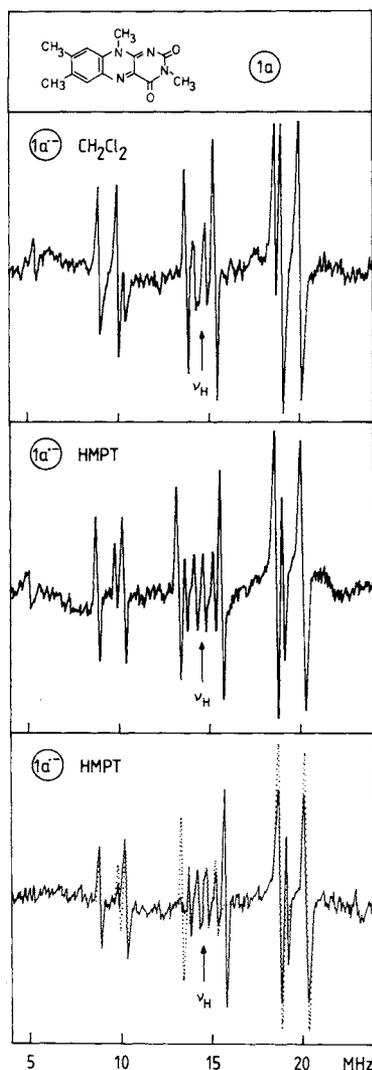
**Figure 5.** ENDOR spectra of the electrochemically generated 3-methylflavin radical anion ( $1a^-$ ) in HMPT and methylene chloride. The general TRIPLE spectrum (HMPT) is also given (bottom spectrum).
