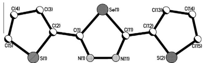
**Figure 3.** Single crystal X-ray structure of compound **5** (hydrogen atoms omitted for clarity). Selected bond lengths (Å) and angles (°) (esds in parentheses): Se(1)–C(1) 1.881(8), Se(1)–C(11) 1.876(8), C(1)–N(1) 1.314(10), C(11)–N(11) 1.300(10), N(1)–N(11) 1.372(9); C(1)–Se(1)–C(11) 81.9(4), Se(1)–C(1)–N(1) 113.6(6), Se(1)–C(11)–N(11) 115.2(7), C(1)–N(1)–N(11) 115.4(7), C(11)–N(11)–N(1) 113.9(7).
