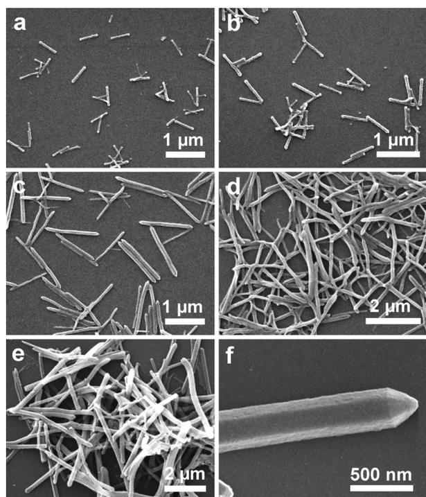
**Fig. 1** SEM images of hexagonal MOF rods with different lengths obtained from Mn(III)-porphyrin **1** and In(NO<sub>3</sub>)<sub>3</sub> at 120 °C at various reaction times; (a) 2, (b) 5, (c) 10, (d) 30, and (e) 60 min, and (f) a magnified image of a MOF rod grown from 60 min of reaction at 120 °C.
