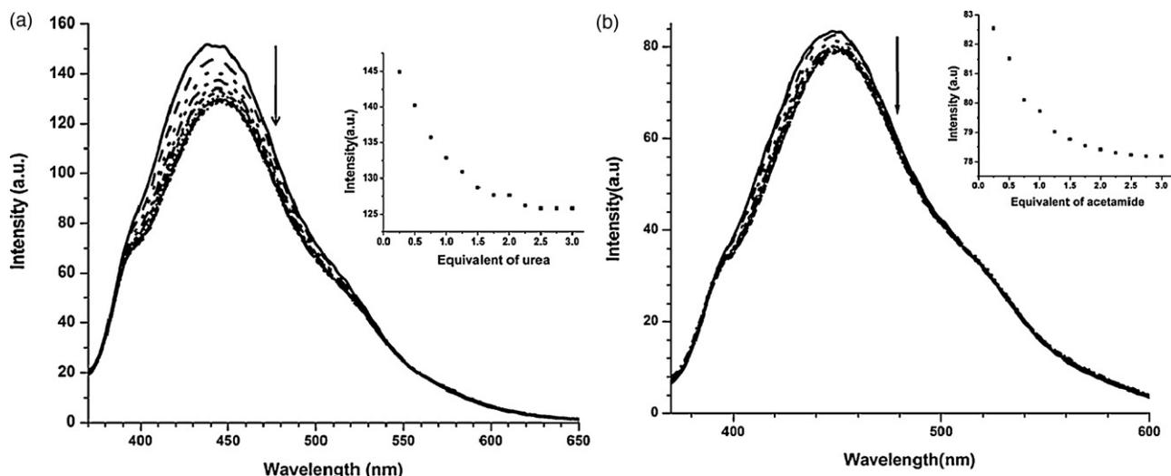
**Fig. 3.** (a) Emission spectra of  $L1 = 10^{-4}$  M in the absence and in the presence of increasing concentrations of urea  $(0-325) \times 10^{-6}$  M. Inset: emission intensity changes upon increasing urea concentrations. (b) Emission spectra of  $L1 = 10^{-4}$  M in the absence and in the presence of increasing concentrations of acetamide  $(0-325) \times 10^{-6}$  M. Inset: emission intensity changes upon increasing acetamide concentrations.
