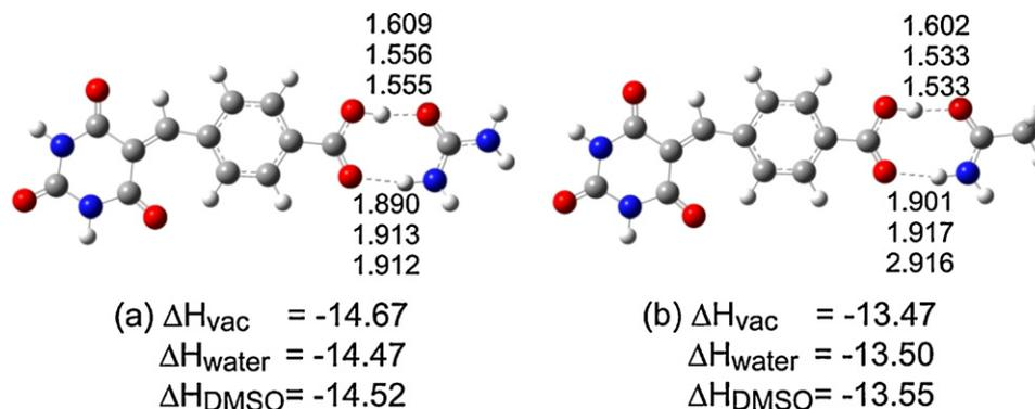
Fig. 6. Optimized structures of L1 with one urea (a) and acetamide (b). The enthalpy changes ( $\Delta H$ ) at 298.15 K ( $\text{kcal mol}^{-1}$ ) of the complexes obtained at the B3LYP/6-31G(d,p) level of theory in gas phase, aqueous and DMSO media are given. Hydrogen bond lengths [ $\text{\AA}$ ] in gas phase, aqueous and DMSO media are given from top to bottom, respectively.
