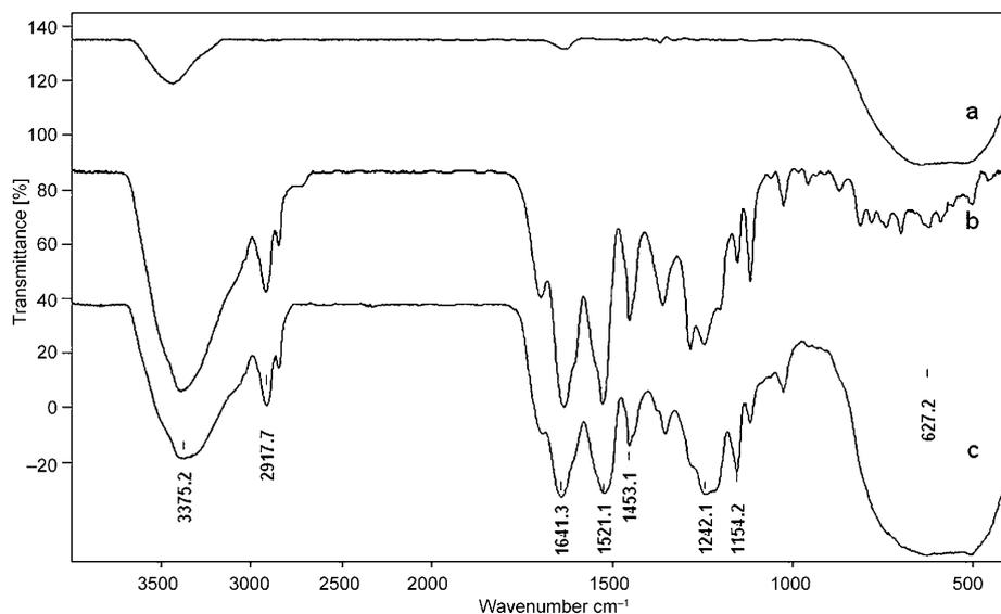
Figure 8. The characteristic FTIR spectrum for a) pure TiO<sub>2</sub> nanoparticles (P25), b) pure triscatecholate **12**, and c) triscatecholate **12** immobilized on TiO<sub>2</sub> nanoparticles.
