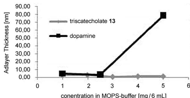
Figure 7. Changes of the adlayer thickness of different concentrations of triscatecholate **13** and dopamine.
