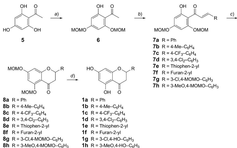
a) ClCH<sub>2</sub>OMe, K<sub>2</sub>CO<sub>3</sub>, acetone, reflux. b) R<sup>1</sup>-CHO, MeOH, NaOH (60% aq.). c) AcONa, EtOH, H<sub>2</sub>O, reflux. d) MeOH, 3M HCl, reflux.
