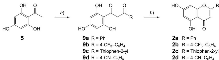
a) RCOCl, K<sub>2</sub>CO<sub>3</sub> (aq.), triethylbenzylammonium chloride (TEBA), benzene, 60°. b) K<sub>2</sub>CO<sub>3</sub> (5% aq.), reflux.
