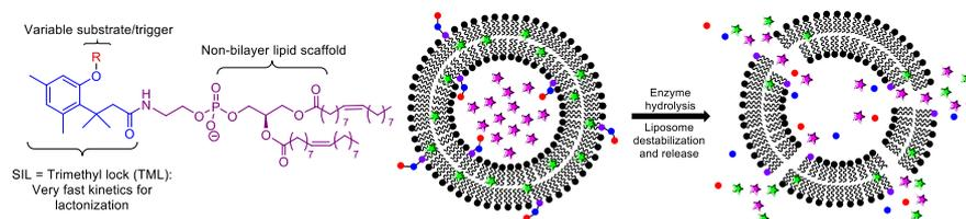
A modular approach is reported for the development of enzyme-responsive liposomes. These exploit synthetic lipid switches containing variable enzyme substrates that, when removed, yield decomposition of a self-immolating linker producing a non-bilayer lipid that perturbs the membrane and triggers release of contents. This approach enables the targeting of a range of enzymes that are overexpressed in diseased cells for drug delivery applications.
