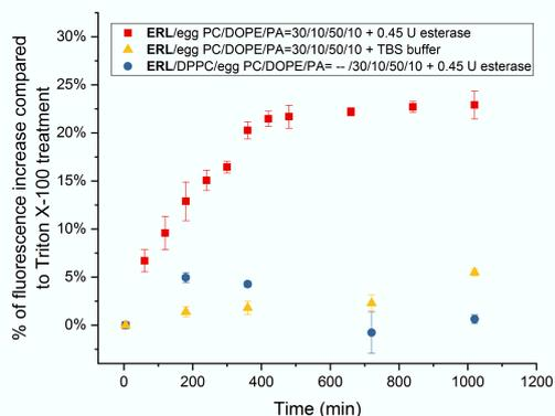
**Figure 3.** SRB release data over time upon esterase addition to liposomes containing 30% **ERL**, 50% DOPE, 10% PC and 10% PA or control experiments of buffer treatment or liposomes lacking **ERL**. Only liposomes containing **ERL** with esterase treatment showed significant fluorescence increases. Error bars indicate standard errors from at least three studies.
