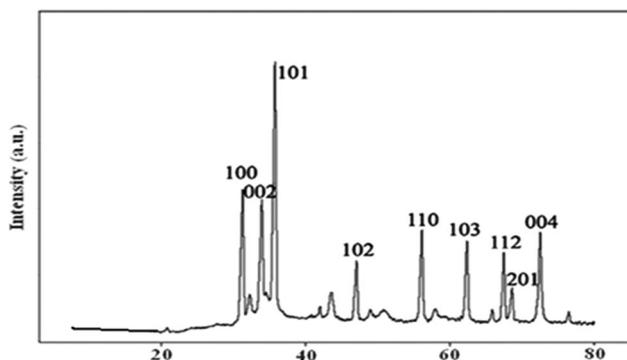
**Fig. 1** XRD pattern of the prepared nanoZnO
