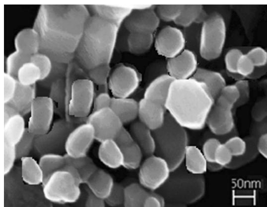
**Fig. 2** The FESEM of the prepared nanoZnO
