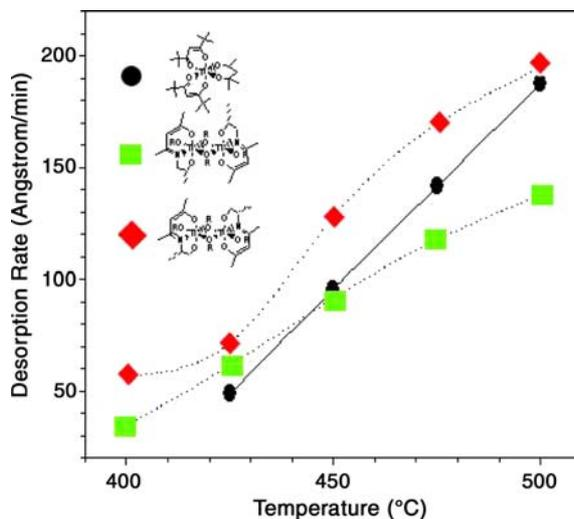
Fig. 4. Deposition rate of TiO<sub>2</sub> layer with several Ti precursors as a function of deposition temperature (deposition conditions(**2b**, **2c**, Ti(mpd)(thd)<sub>2</sub>) solvent: *n*-butyl acetate (0.05 M, 5 ml), *n*-butyl acetate (0.05 M, 3 ml), MeOH (0.05 M, 5 ml); temperature of evaporation: 260, 230, 260 °C; temperature of substrate: 400–500 °C).
