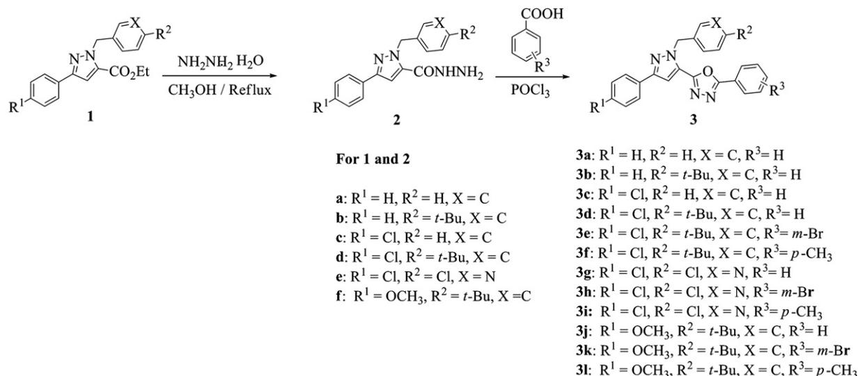
Fig. 1. Synthesis of substituted pyrazolopyridazine derivatives.
