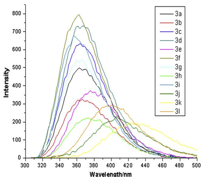
Fig. 7. The Fluorescence spectra of the compounds **3a–l** in dichloromethane ( $2 \times 10^{-6}$  M).
