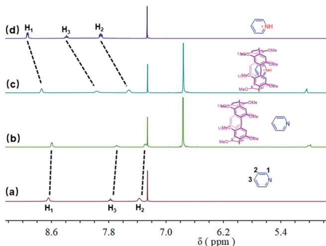
Figure 1. Partial <sup>1</sup>H NMR spectra (400 MHz, CDCl<sub>3</sub>, 298 K): (a) 5.00 mM **pyridine**; (b) 5.00 mM **pyridine** + 5.00 mM **MeP5A**; (c) 5.00 mM **pyridine** + 10.00 mM **TFA** + 5.00 mM **MeP5A**; (d) 5.00 mM **pyridine** + 10.00 mM **TFA**.
