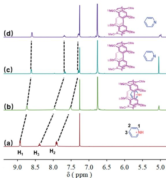
Figure 2. Partial <sup>1</sup>H NMR spectra (400 MHz, CDCl<sub>3</sub>, 298 K): (a) 5.00 mM **pyridine** + 10.00 mM **TFA**; (b) 5.00 mM **pyridine** + 5.00 mM **MeP5A** + 10.00 mM **TFA**; (c) 5.00 mM **pyridine** + 5.00 mM **MeP5A** + 10.00 mM **TFA** + 15.00 mM *i*Pr<sub>2</sub>NEt; (d) 5.00 mM **pyridine** + 5.00 mM **MeP5A**.
