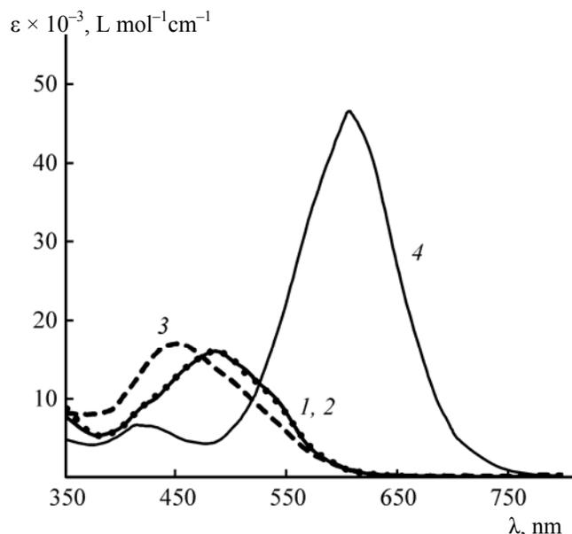
**Fig. 1.** Electronic absorption spectra of (1, 2) formazan **2** and (3, 4) formazan **5** at (1, 3) pH 6 and (2, 4) 12.
