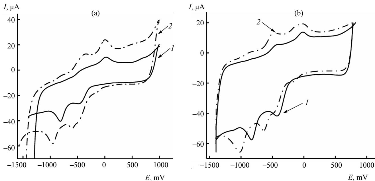
**Fig. 2.** Cyclic voltammograms of formazans (a, 1) **2** and (a, 2) **5** and tetrazolium betaines (b, 1) **3** and (b, 2) **6**.
