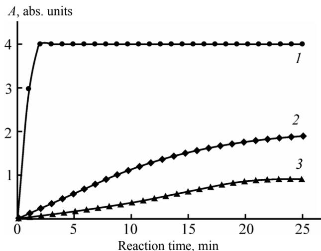
**Fig. 3.** Plots of optical density against time for solutions of tetrazolium salts (1) **6**, (2) **3**, and (3) 2,3,5-triphenyl-2*H*-tetrazolium chloride in the course of reduction with sodium sulfide.
