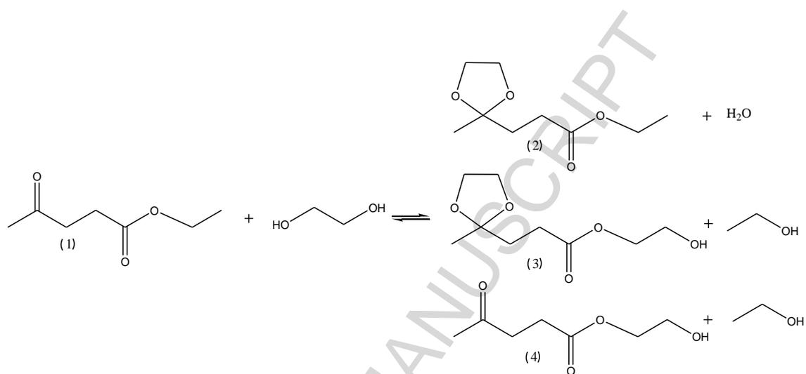
**Fig. 1.** Ketalization reaction between ethyl levulinate (EL) and ethylene glycol (EG).
