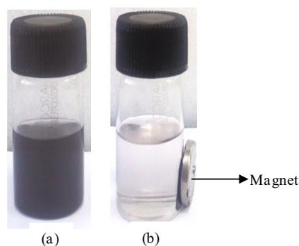
**Fig. 9.** Dispersion of CoFe<sub>2</sub>O<sub>4</sub> nanoparticles in water-ethanol 1:1 mixture (a) and magnetic separation of catalyst (b).
