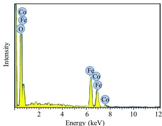
Fig. 3. EDX analysis of  $\text{CoFe}_2\text{O}_4$  nanoparticles.
