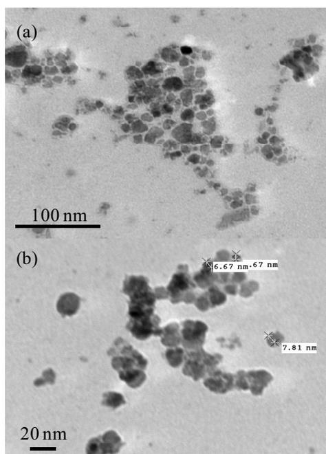
Fig. 5. TEM images of CoFe<sub>2</sub>O<sub>4</sub> nanoparticles.
