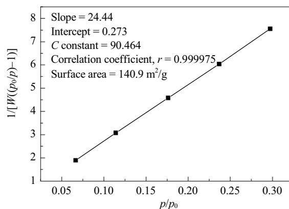
Fig. 7. BET plot of CoFe<sub>2</sub>O<sub>4</sub> nanoparticles.
