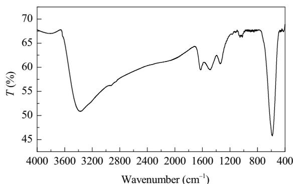
Fig. 1. FT-IR spectrum of  $\text{CoFe}_2\text{O}_4$  nanoparticles.
