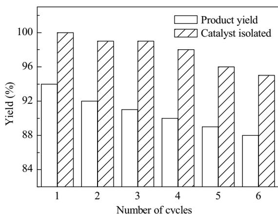
Fig. 10. The recyclability of CoFe<sub>2</sub>O<sub>4</sub> nanoparticles for synthesis of 3a.
