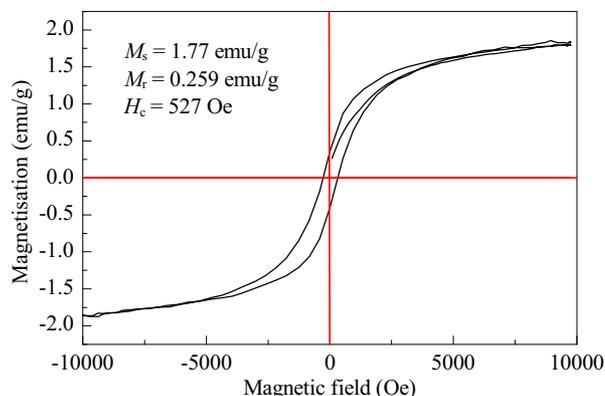
Fig. 6. Field-dependent magnetization of CoFe<sub>2</sub>O<sub>4</sub> nanoparticles.
