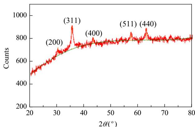
Fig. 2. XRD pattern of  $\text{CoFe}_2\text{O}_4$  nanoparticles.
