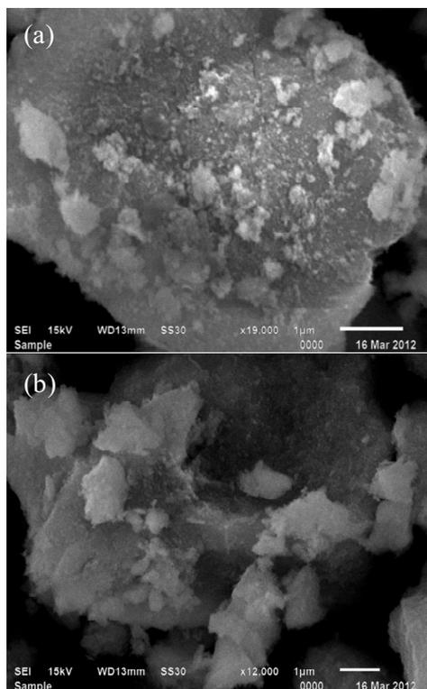
Fig. 4. SEM images of CoFe<sub>2</sub>O<sub>4</sub> nanoparticles.
