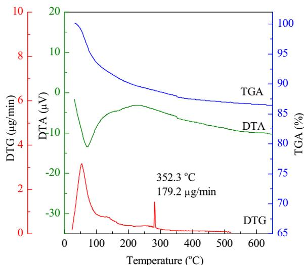
Fig. 8. TGA/DTA/DTG analysis of  $\text{CoFe}_2\text{O}_4$  nanoparticles.
