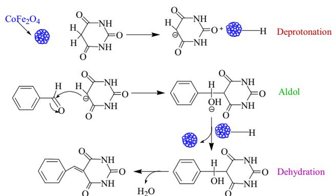
**Scheme 1.** Proposed mechanism for synthesis of arylidene barbituric acid **3a** using CoFe<sub>2</sub>O<sub>4</sub> nanocatalyst.
