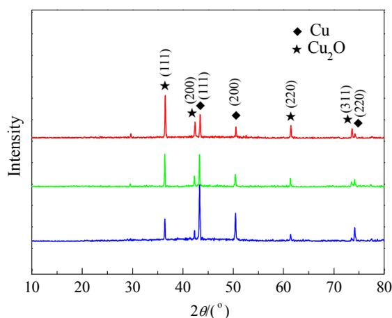
**Fig. 4.** XRD patterns of PdCl<sub>2</sub>/Cu-Cu<sub>2</sub>O catalysts synthesized with varying amounts of glucose. (1) 10 mmol; (2) 15 mmol; (3) 20 mmol.
