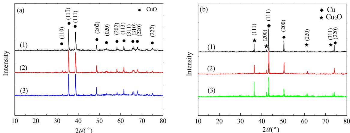
**Fig. 1.** XRD patterns of PdCl<sub>2</sub>/CuO (a) and PdCl<sub>2</sub>/Cu-Cu<sub>2</sub>O (b) catalysts synthesized using various NaOH concentrations. (1) 2.5 mol/L; (2) 5 mol/L; (3) 10 mol/L.
