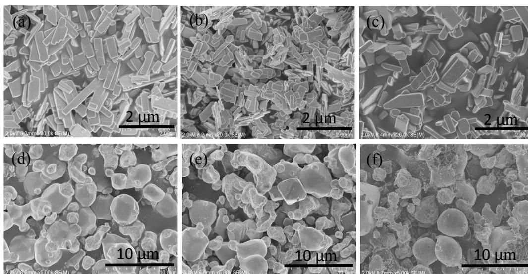
**Fig. 3.** SEM images of PdCl<sub>2</sub>/CuO (a–c) and PdCl<sub>2</sub>/Cu-Cu<sub>2</sub>O (d–f) catalysts synthesized at various NaOH concentrations. (a, d) 2.5 mol/L; (b, e) 5 mol/L; (c, f) 10 mol/L.
