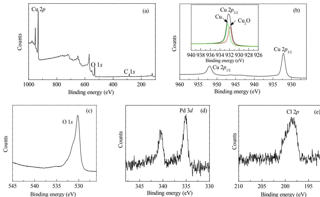
Fig. 7. (a) The complete XPS spectrum and the high-resolution XPS spectra for the (b) Cu 2p, (c) O 1s, (d) Pd 3d and (e) Cl 2p regions for PdCl<sub>2</sub>/Cu-Cu<sub>2</sub>O catalysts made with 10 mmol glucose.
