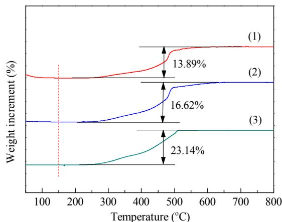
**Fig. 5.** TG data for PdCl<sub>2</sub>/Cu-Cu<sub>2</sub>O catalysts synthesized with varying amounts of glucose. (1) 10 mmol; (2) 15 mmol; (3) 20 mmol.
