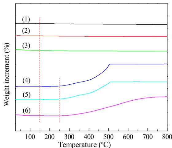
**Fig. 2.** TG patterns of PdCl<sub>2</sub>/CuO (1–3) and PdCl<sub>2</sub>/Cu-Cu<sub>2</sub>O (4–6) catalysts synthesized using different NaOH concentrations. (1, 4) 2.5 mol/L; (2, 5) 5 mol/L; (3, 6) 10 mol/L.
