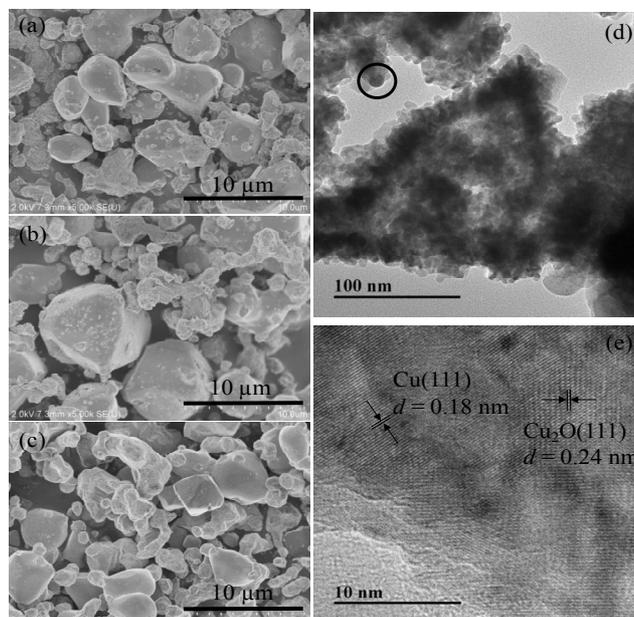
**Fig. 6.** SEM images of PdCl<sub>2</sub>/Cu-Cu<sub>2</sub>O catalysts synthesized with varying amounts of glucose. (a) 10 mmol; (b) 15 mmol; (c) 20 mmol. TEM (d) and HRTEM (e) images of the PdCl<sub>2</sub>/Cu-Cu<sub>2</sub>O catalyst synthesized using 10 mmol glucose.
