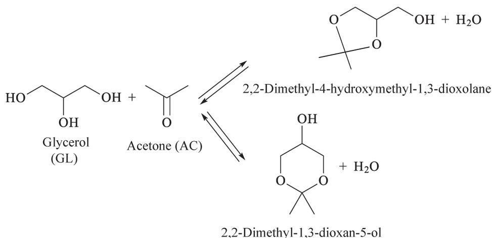
Experiments on the solketal synthesis from crude glycerol were performed in a 500-mL three-necked flask equipped with a thermometer, a reflux condenser, and a power-driven controllable-rate stirrer. The experiments were performed at 20–25°C; the stirrer rotation rate was 1500 rpm. Acetone was added in a 3–6.5-fold molar excess relative to glycerol.
