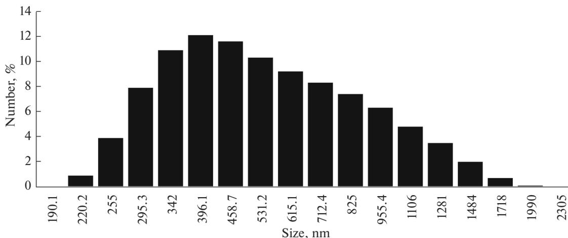
**Fig. 3.** Grain size distribution of synthesized thorite with DLS.
