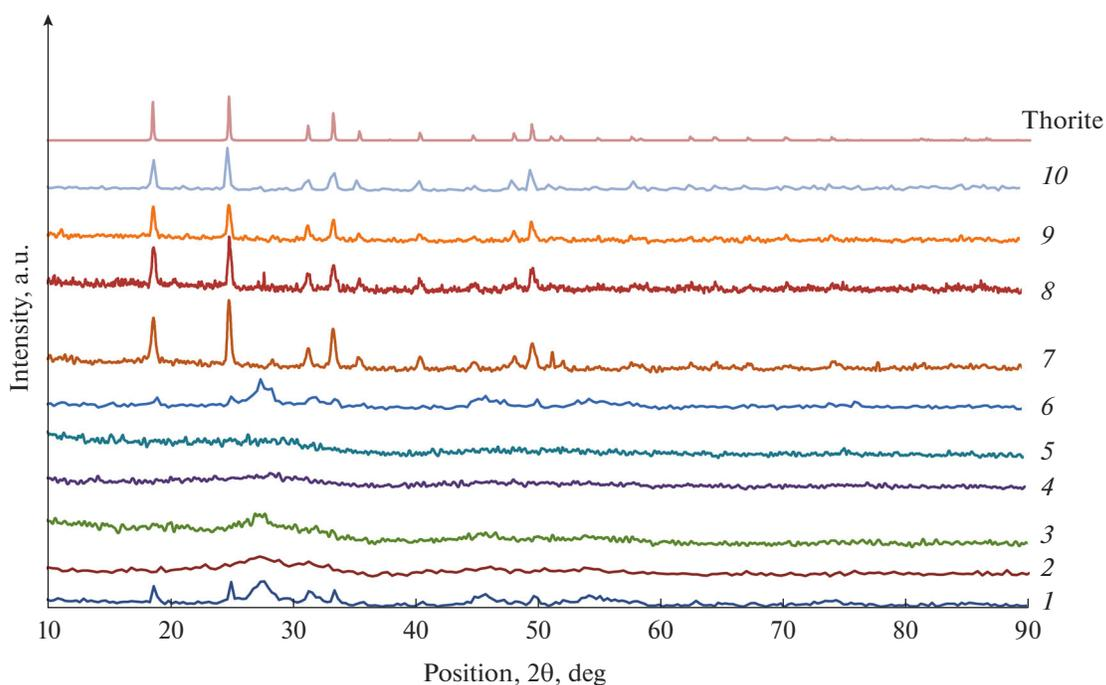
Fig. 1. XRD diagrams of 10 synthesized products compared with thorite ( $\text{ThSiO}_4$ ).
