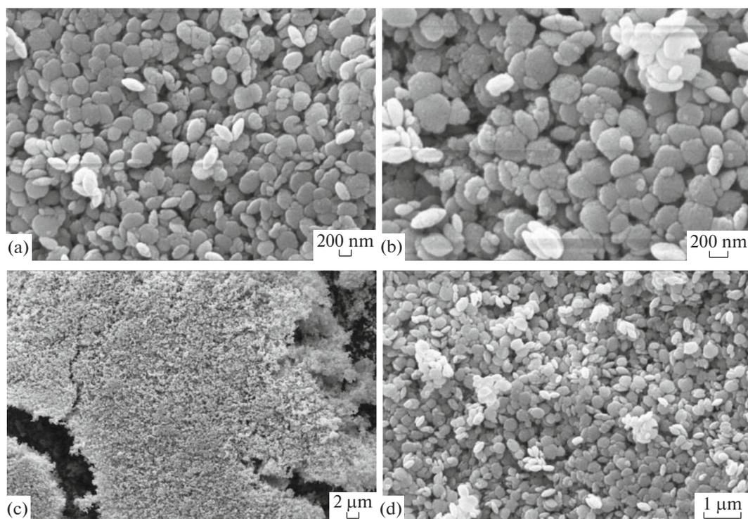
Fig. 2. SEM observations of synthetic thorite.
