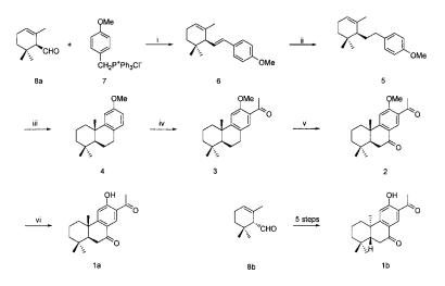
Reagents and conditions: i) n-BuLi, n-hexane, r.t., 5h (70%); ii) 5% Pd/C, ethanol (95%); iii) BF<sub>3</sub>·Et<sub>2</sub>O, CH<sub>2</sub>Cl<sub>2</sub>, 12 h (93%); iv) acetyl chloride, anhydrous AlCl<sub>3</sub>, -5°C, 2h, (90%); v) CrO<sub>3</sub>/HOAc/H<sub>2</sub>O, r.t., 0.5h (90%); vi) anhydrous AlCl<sub>3</sub>, CH<sub>2</sub>Cl<sub>2</sub>, r.t., 8 h (95%).
