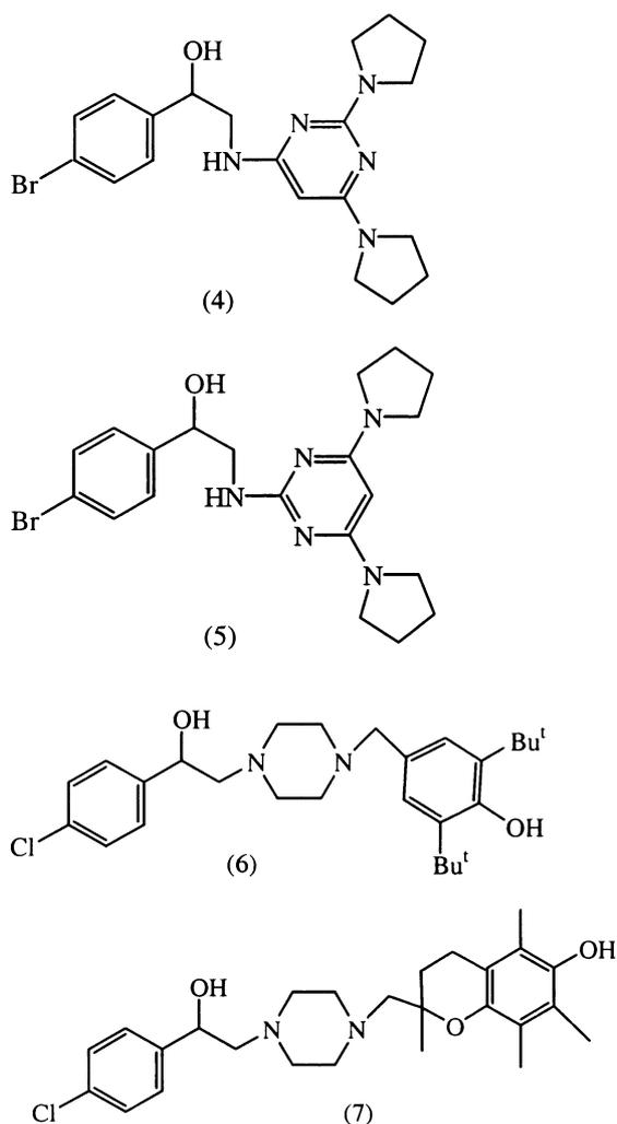
pyrimidines (9a–c). Reaction with piperazine at 120°C in a Carius tube using pyridine as a solvent gave (10a–c) in superior yields to those reported using milder reaction conditions.<sup>[8]</sup> Reaction with  $\alpha$ -bromo-*p*-bromoacetophenone followed by reduction of the intermediate ketones (11) gave the target amino alcohols (3a–c).
