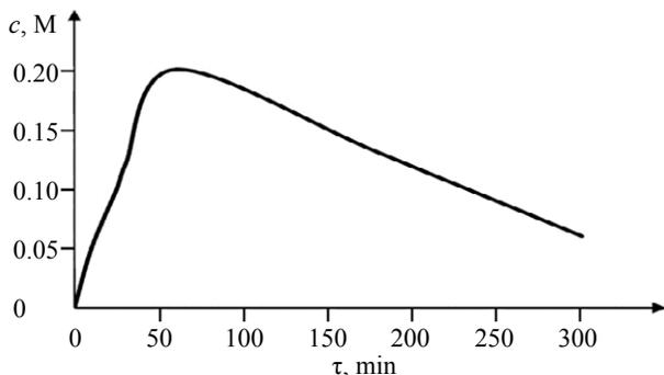
Fig. 2. Kinetic curve for the accumulation of 4-methyl-4-phenyl-1,3-dioxane (**3**) in the reaction of  $\alpha$ -methylstyrene with formaldehyde and methylamine hydrochloride (100°C); initial concentrations, M: [I] = 3.33, [MeNH<sub>2</sub>·HCl] = 3.33, [CH<sub>2</sub>O] = 6.66.
