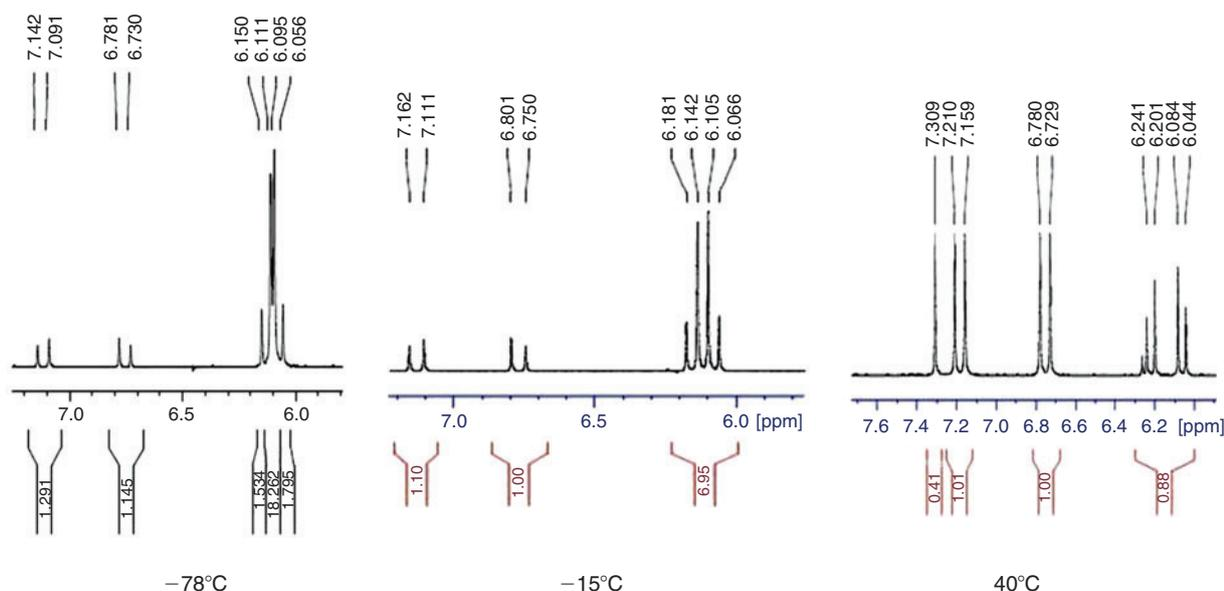
Fig. 1. Part of the  $^1\text{H}$  NMR spectra of the products formed from the reaction of 1-methylpiperazine with maleic anhydride at different temperatures.
