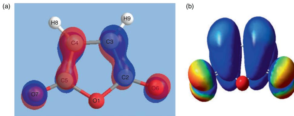
Fig. 3. (a) LUMO and (b) electrostatic potential map of the maleic anhydride molecule.
