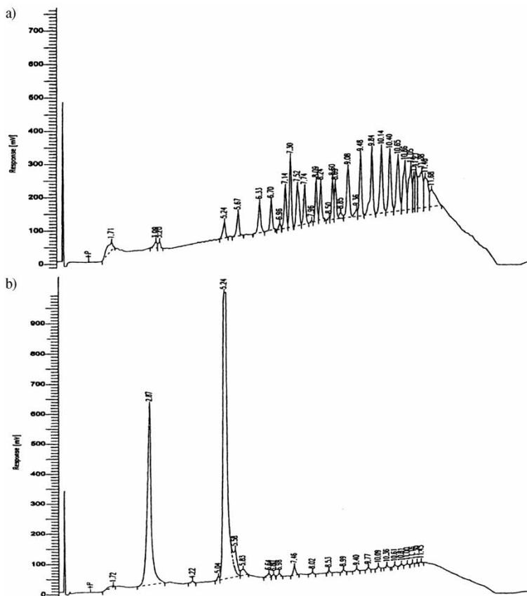
**Figure 2.** (top) HPLC trace of oligosalicylate, (bottom) HPLC trace following reaction with amine. The peak on the left is salicylic acid and the peak on the right is product.
