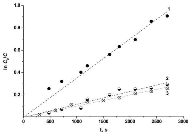
**Figure 4.** Kinetic dependences of DTC oxidation ( $c\ 2.6 \times 10^{-3}$  M) in presence of homogeneous phthalocyanine catalysts ( $c\ 5.6 \times 10^{-5}$  M) (1) Co(NH)Pc6, (2) Co(O)Pc4, (3) Co(S)Pc5 in water-alkali solution (pH 11) at 298.15 K. The dotted line: the result of the formal processing of the kinetic equation
