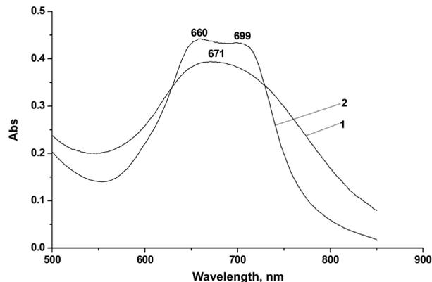
**Figure 2.** UV-vis spectra of Co(X)Pc ( $c 5.5 \times 10^6$  M) in NH<sub>4</sub>OH 5% aqueous solution: (1) Co(O)Pc4, (2) Co(S)Pc5 at 298.15 K
