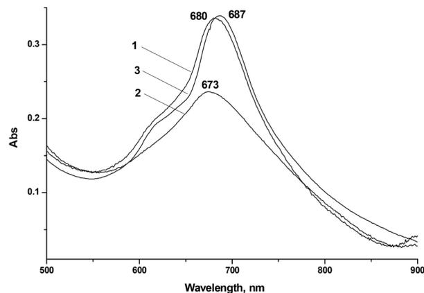
**Figure 1.** UV-vis spectra of Co(X)Pc ( $c 4.5 \times 10^{-6}$  M) in DMF: (1) Co(O)Pc4, (2) Co(S)Pc5, (3) Co(NH)Pc6 at 298.15 K
