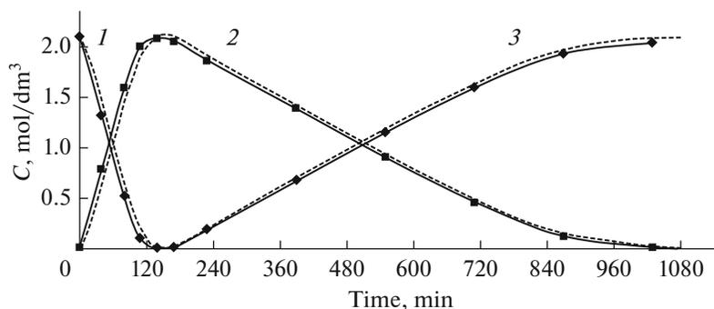
**Fig. 6.** Kinetics of the consumption and accumulation of products in dicyclopentadiene hydrogenation: (---) calculated and (—) experimental vdata; (1) dicyclopentadiene, (2) dicyclopentene, and (3) dicyclopentane. The solvent is toluene,  $C_{\text{cat}} = 4$  g/dm<sup>3</sup>, and  $T = 338$  K.
