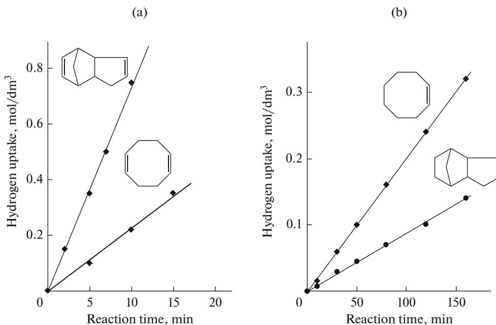
**Fig. 3.** Effect of the nature of cycloolefin on the reactivity of its double bonds in (a) diene and (b) monoolefin hydrogenation. The solvent is toluene,  $C_{\text{cat}} = 4 \text{ g/dm}^3$ ,  $T = 338 \text{ K}$ , and  $C^0 = 1.04 \text{ mol/dm}^3$ .
