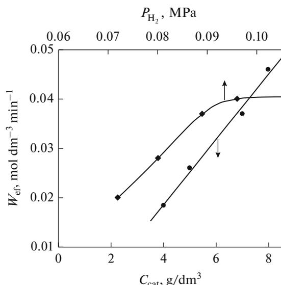
**Fig. 5.** Hydrogen uptake rate in dicyclopentadiene hydrogenation as a function of the catalyst concentration and hydrogen partial pressure. The solvent is toluene,  $T = 333$  K, and  $C_{\text{DCPD}}^0 = 1.04$  mol/dm<sup>3</sup>.
