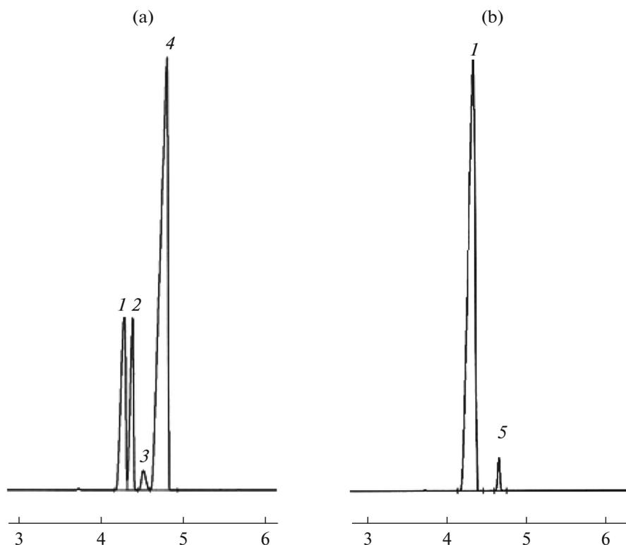
**Fig. 2.** Chromatogram of products of (a) complete and (b) partial 1,5-*cis,cis*-cyclooctadiene hydrogenation to *cis*-cyclooctene. (1) Cyclooctene, (2, 3) intermediate products, (4) cyclooctadiene, and (5) cyclooctane.
