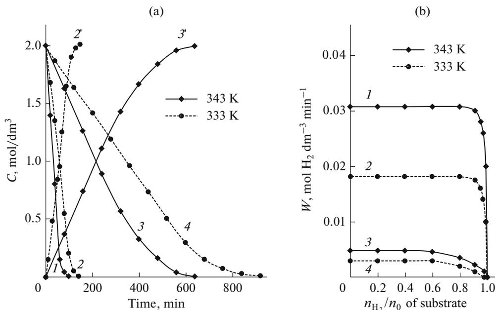
**Fig. 4.** (a) Kinetics of substrate consumption during the hydrogenation of (1, 2) dicyclopentadiene to dicyclopentene and (3, 4) dicyclopentene to dicyclopentane and the kinetics of accumulation of (2') dicyclopentene and (3') dicyclopentane. (b) Reaction rate depending on the reaction temperature. The solvent is toluene,  $C^0 = 2.0 \text{ mol/dm}^3$ , and  $C_{\text{cat}} = 4 \text{ g/dm}^3$ .
