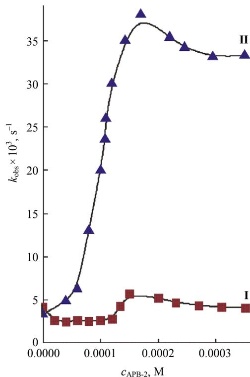
**Fig. 4.** Plots of the observed rate constant of alkaline hydrolysis of phosphonates **I** and **II** versus concentration of APB-2; 0.001 M NaOH, 25°C.
