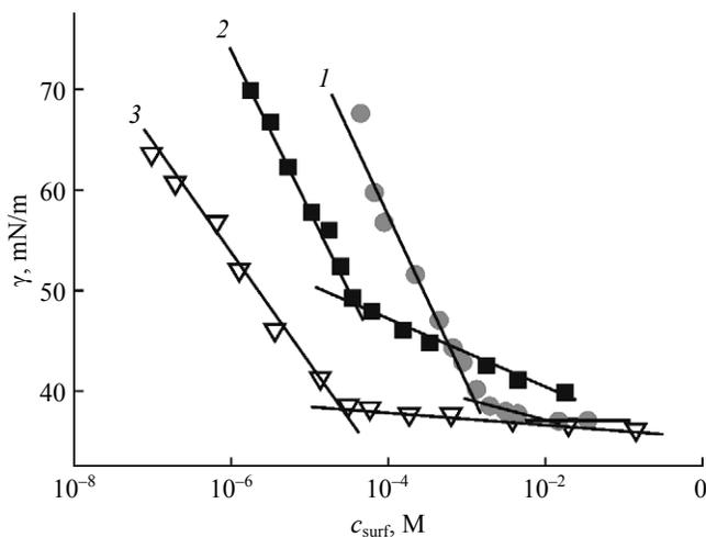
**Fig. 1.** Surface tension isotherms of aqueous solutions of (1) APB-1 and (2) APB-2 and (3) of binary system APB-2–polyethylenimine;  $c_{\text{PEI}} = 0.05 \text{ M}$ ,  $25^\circ\text{C}$ .
