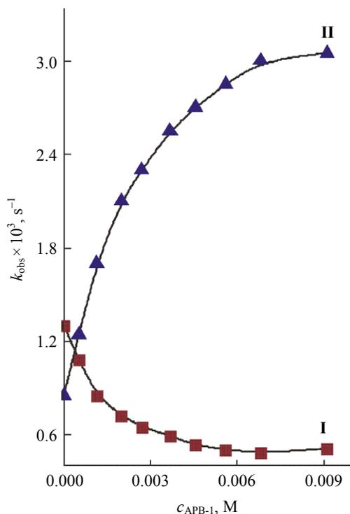
**Fig. 5.** Plots of the observed rate constant of alkaline hydrolysis of phosphonates **I** and **II** versus concentration of APB-1 in the binary system APB-1–polyethylenimine,  $c_{\text{PEI}} = 0.05 \text{ M}$ ,  $25^\circ\text{C}$ .
