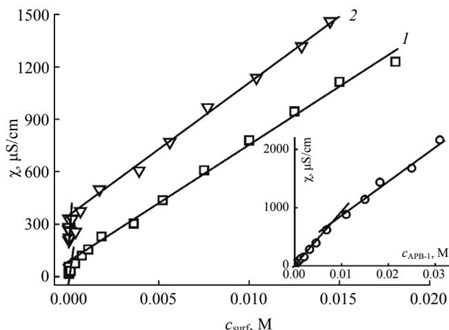
**Fig. 2.** Plots of the specific electrical conductivity of (1) aqueous solution of APB-2 and (2) binary system APB-2–polyethylenimine versus surfactant concentration;  $c_{PEI} = 0.05$  M, 25°C. The corresponding dependence for APB-1 is shown in the insert.
