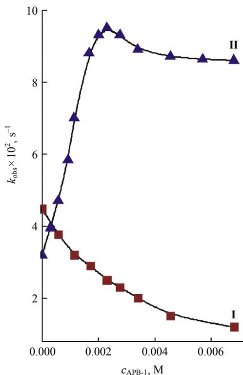
**Fig. 3.** Plots of the observed rate constant of alkaline hydrolysis of phosphonates **I** and **II** versus concentration of APB-1; 0.01 M NaOH, 25°C.
