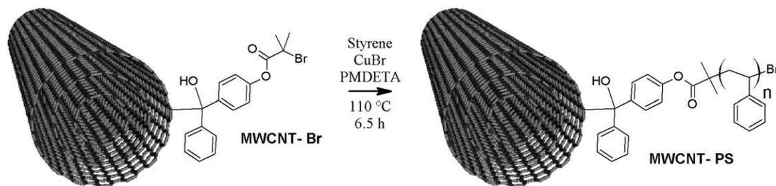
**SCHEME 2** ATRP of styrene from the initiator functionalized MWCNT-Br. TGA of such a sample is shown in Figure 2, where A is Sigma-Aldrich and B is Nanocyl.
