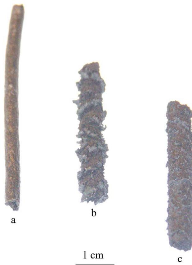
**FIGURE 5** Extruded samples of a standard PPS (a), a PPS composite with pristine MWCNT (b) and a PPS composite with MWCNT-PS (c).
