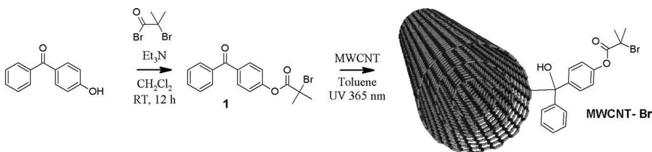
**SCHEME 1** Preparation of the UV sensitive ATRP initiator and subsequent reaction with MWCNTs under UV irradiation at 365 nm.
