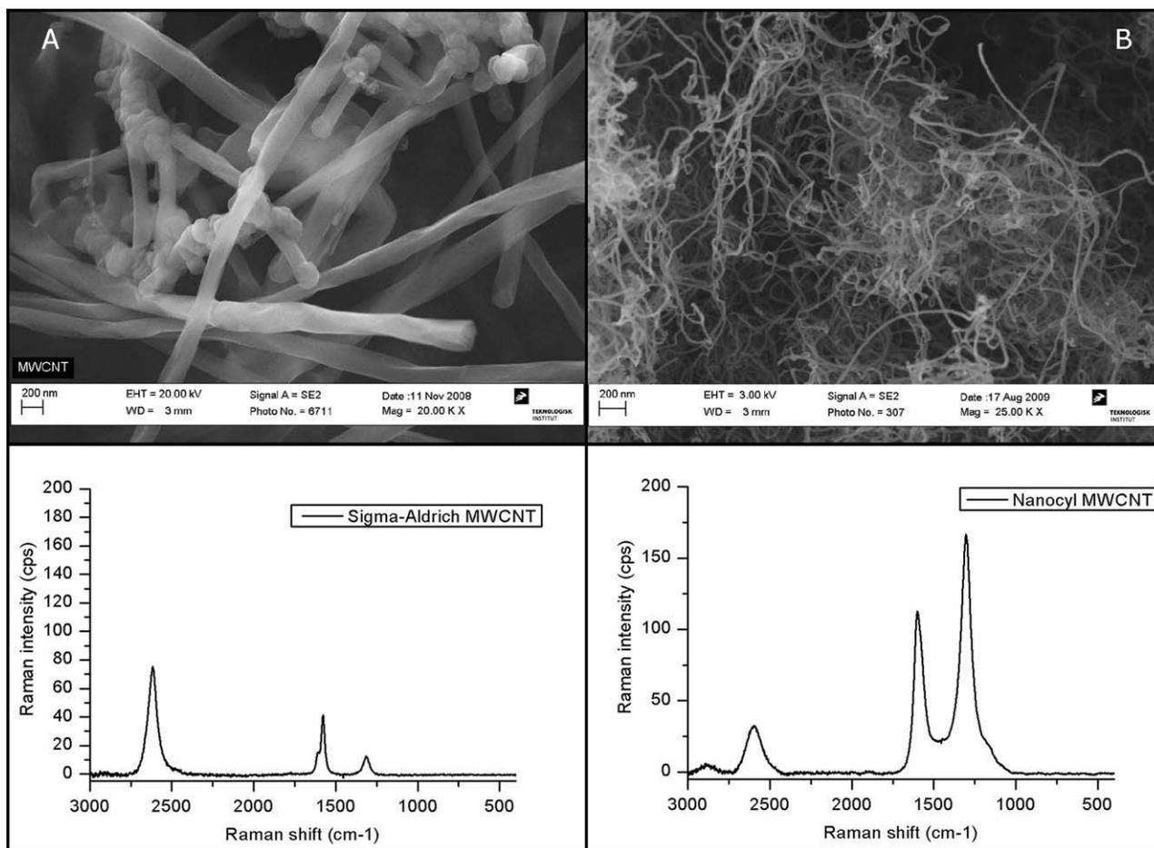
**FIGURE 1** Raman spectra and scanning electron micrographs of the two different grades of MWCNT. The left column shows data on the pristine MWCNT from Sigma-Aldrich (A), the right column shows data on the pristine MWCNT from Nanocyl (B).
