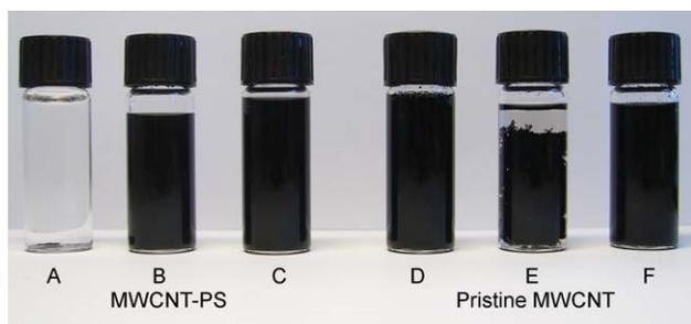
**FIGURE 4** Dispersion experiments of MWCNT-PS (Nanocyl, A-C) compared with pristine MWCNT (Nanocyl, D-F) 1.5 h after dispersion. The dispersions have been prepared at 20 °C in cyclohexane (A,D), dichloromethane (B,E), and dioxane (C,F) with a concentration of 0.5 mg/mL.
