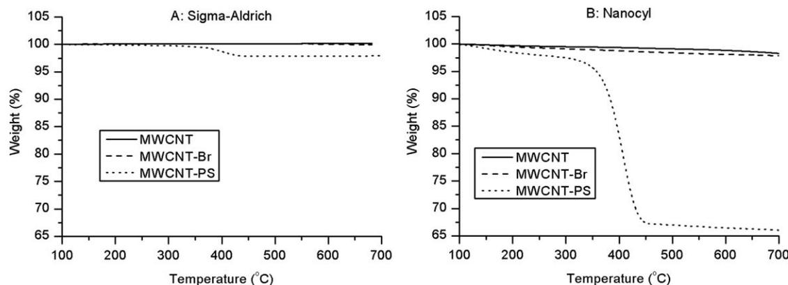
**FIGURE 2** TGA analyses of the two grades of MWCNT before and after introduction of the initiator and subsequent ATRP of styrene.
