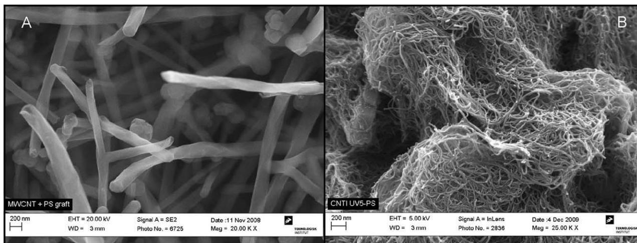
**FIGURE 3** Scanning electron micrographs of polystyrene-grafted MWCNT, A: Sigma-Aldrich MWCNT-PS, B: Nanocyl MWCNT-PS.
