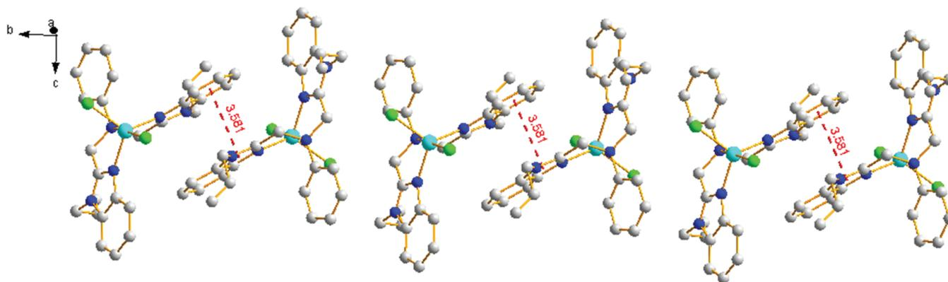
Fig. 4 The  $\pi\cdots\pi$  interactions and packing modes in complex 4 (H atoms are omitted).
