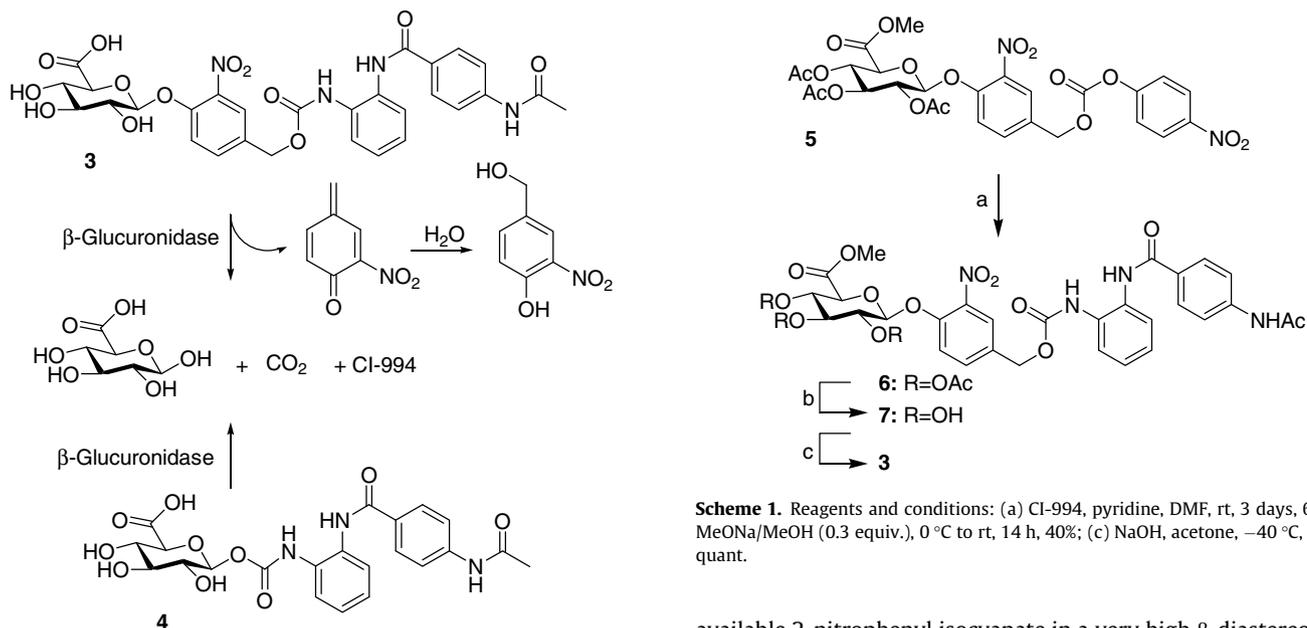
Scheme 1. Reagents and conditions: (a) CI-994, pyridine, DMF, rt, 3 days, 60%; (b) MeONa/MeOH (0.3 equiv.), 0 °C to rt, 14 h, 40%; (c) NaOH, acetone, −40 °C, 15 min, quant.
