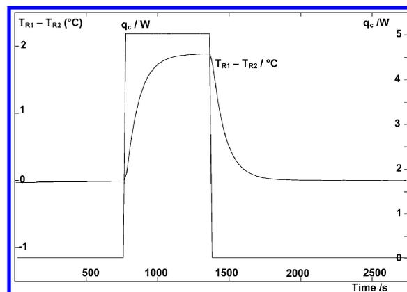
**Figure 4.** Calibration of the differential reaction calorimeter by Joule effect.
