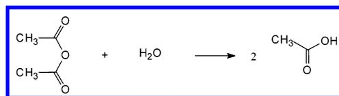
**Figure 5.** Reaction scheme of the hydrolysis of acetic anhydride.
