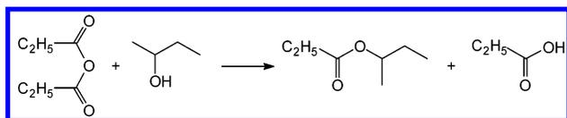
**Figure 7.** Reaction scheme of the esterification of acetic anhydride by 2-butanol.
