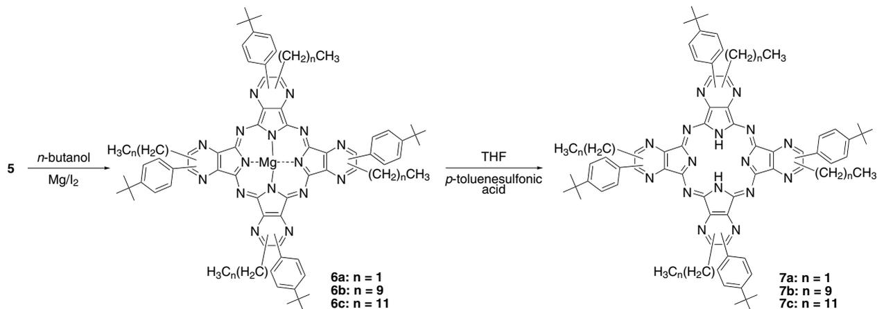
**Scheme 2.** Reaction route of the magnesium and metal-free tetrapyrazinoporphyrazine complexes
