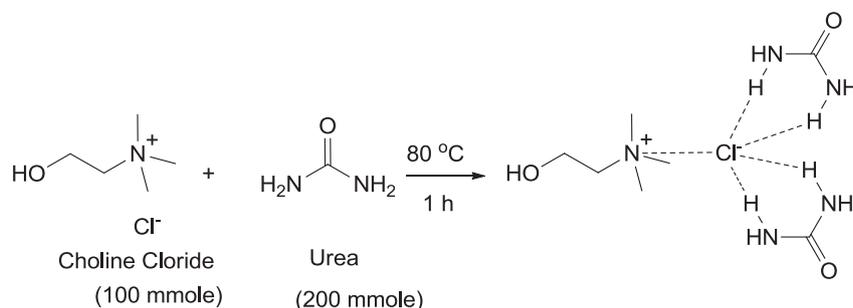
Fig. 1. Deep eutectic solvent preparation.
