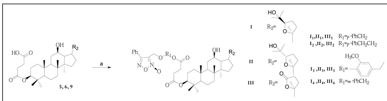
Scheme 3: Synthesis of final products (compounds **I**<sub>1-4</sub>, **II**<sub>1-4</sub>, **III**<sub>1-4</sub>) *Reagents and conditions:* a) **A**<sub>1.4</sub>, DMAP, EDCI,  $25^\circ\text{C}$ ,  $\text{CH}_2\text{Cl}_2$ , 6 h.
