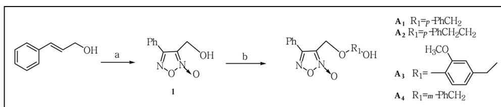
Scheme 1: Synthesis of furoxans **A**<sub>1-4</sub> Reagents and conditions: a) NaNO<sub>2</sub>, HOAc, r.t., 1 h; b) (i) SOCl<sub>2</sub>, pyridine, CH<sub>2</sub>Cl<sub>2</sub>, r.t., 8 h; (ii) HOR<sub>1</sub>OH, K<sub>2</sub>CO<sub>3</sub>, KI, CH<sub>3</sub>CN, r.t., 3 h.
