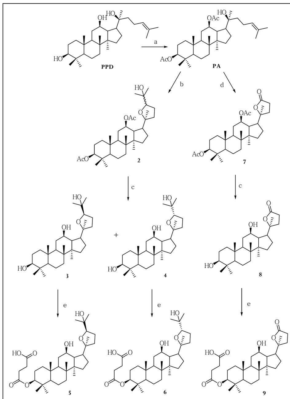
Scheme 2: Synthesis of the derivatives from **PPD** (compounds **5, 6, 9**) *Reagents and conditions:* a)  $(\text{CH}_3\text{CO})_2\text{O}$ , DMAP,  $\text{CHCl}_3$ , r.t., 12 h; b) *m*-CPBA,  $\text{CH}_2\text{Cl}_2$ ,  $-3^\circ\text{C}$ , 5 h; c)  $\text{NaOH}$ ,  $\text{H}_2\text{O}$ ,  $\text{CH}_3\text{OH}$ , reflux, 6 h; d)  $\text{CrO}_3$ ,  $\text{CH}_3\text{COOH}$ ,  $\text{H}_2\text{O}$ , r.t., 3 h; e) Succinic anhydride, DMAP,  $\text{CHCl}_3$ ,  $42^\circ\text{C}$ , 6 h.
