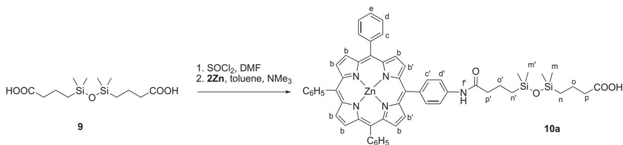
**Scheme 3.** Amide coupling reaction of **2Zn** with the carboxylate-functionalized siloxane **9**
