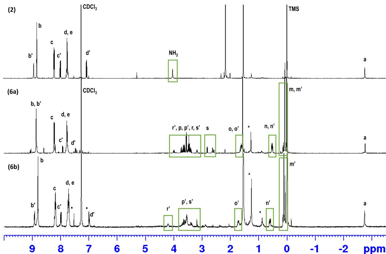
**Fig. 1.**  $^1\text{H}$  NMR spectra in  $\text{CDCl}_3$  of 5-(4-aminophenyl)-10,15,20-triphenylporphyrin (**2**) and of porphyrin mono- (compound **6a**) and disubstituted (compound **6b**); \* denote solvent peaks (hexane in the spectra of **6a** and **6b**); • are satellites
