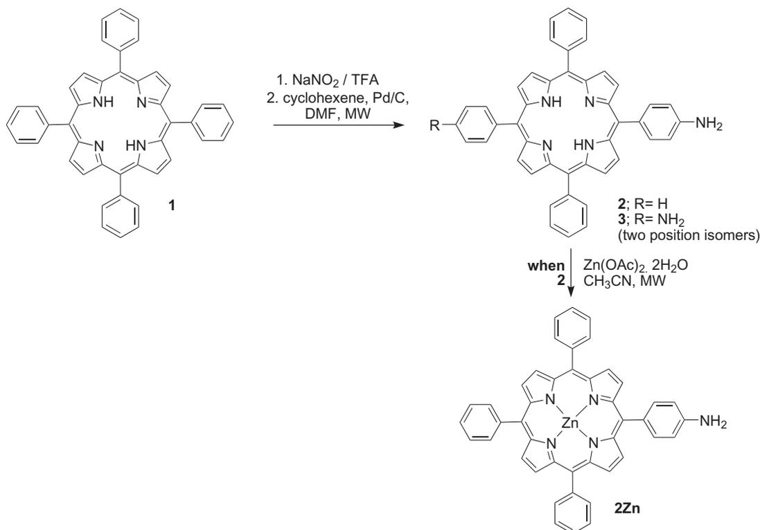
Scheme 1. Microwave-assisted synthesis of amino-functionalized porphyrins and Zn(II) complex
