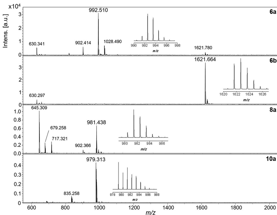
**Fig. 2.** Positive ion mode MALDI-TOF mass spectra of compounds **6a**, **6b**, **8a** and **10a**. Graphical insets display the isotopic patterns observed for the  $MH^+$  ions of compounds **6a**, **6b** and **8a**, and the  $M^+$  ion of compound **10a**
