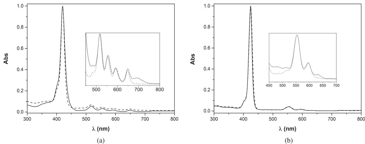
**Fig. 3.** Absorption spectra of: (a) compound **6b** (solid line) and **2** (dashed line) and (b) compound **10a** (solid line) and **2Zn** (dashed line) in chloroform. Zoom of the corresponding Q bands was inserted
